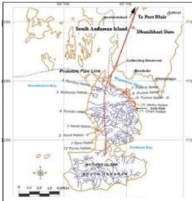
Figure-9.5.1 Plan of Interisland transfer of spring water from Rutland
