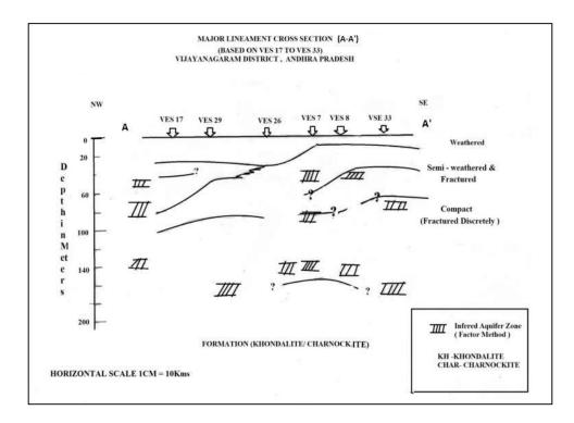
Fig.2.12: Geo-electrical section along A-A'
