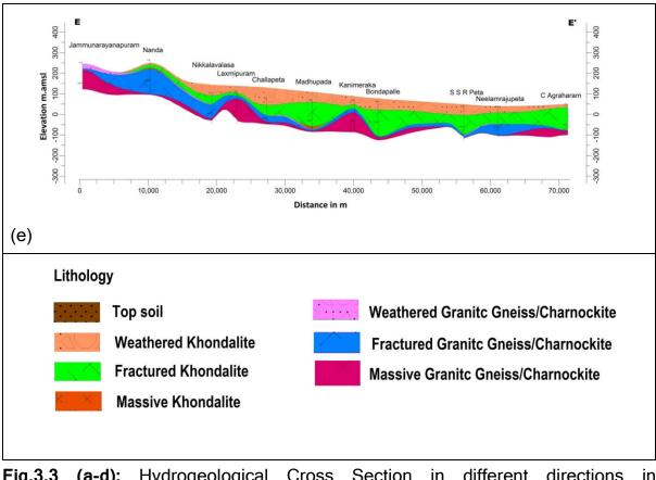
**Fig.3.3 (a-d):** Hydrogeological Cross Section in different directions in Vizianagaram district.
