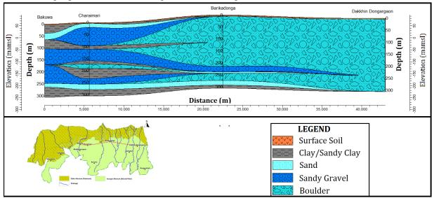
Fig 3.1.1: Section Diagram of Dakkhin Dongargaon- Bakuwa Section
