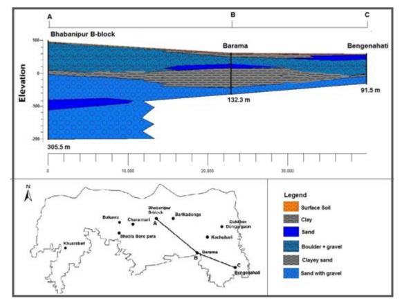
Fig 3.1.2: Section of Bhabanipur B-Block - Bengenahati Section
