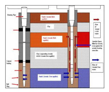
Fig.6.3: Tube-well design of a deep tube well tapping safe deeper aquifer
