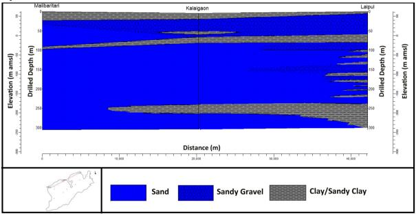
Fig.3.2: Section showing aquifer disposition along northern part
