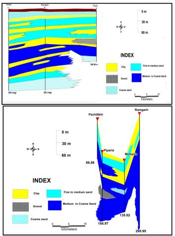
Fig: Aquifer disposition along Ramgarh block
