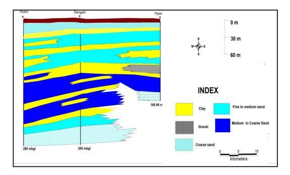
Fig: Aquifer disposition along Nuaon block
