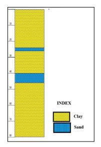
Fig: Lihtological log of exploratory well at Chainpur block.
