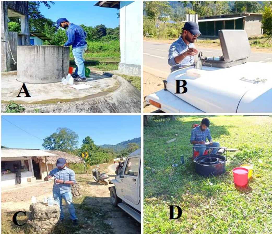
Fig: 2.2.(A) Measuring Ground Water level and (B) In-situ measurement chemical parameter by water quality testing kit (C) Collection of water sample and (D) Conducting Soil Infiltration test
