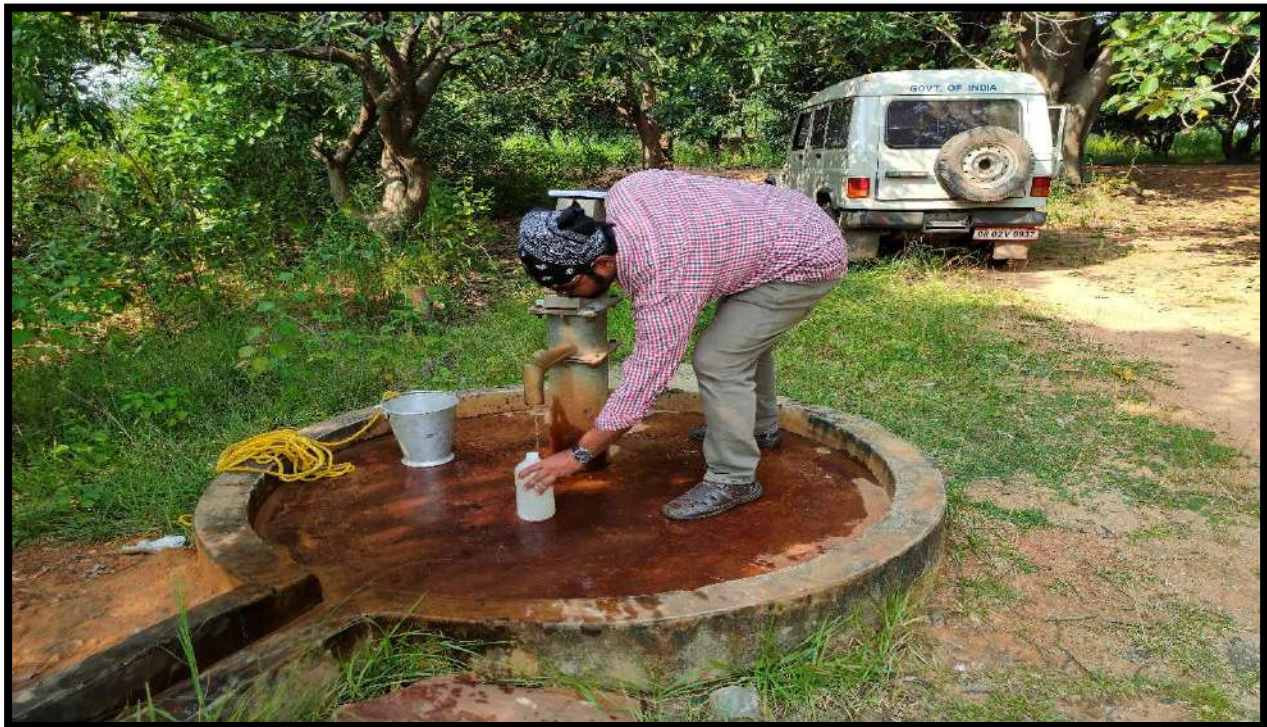
Photograph 2- Chemical sampling from Handpumps
