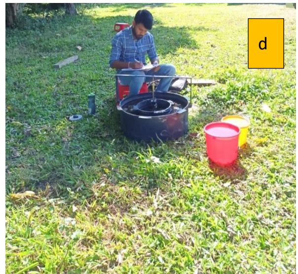
Fig 2.2: (a) Measuring of water level from dug well (b) measuring of in-situ chemical parameter by water quality testing kit (c) Collection of water sample (d) Soil infiltration test.
