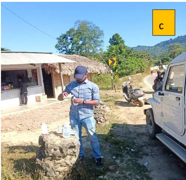
Fig 2.2: (a) Measuring of water level from dug well (b) measuring of in-situ chemical parameter by water quality testing kit (c) Collection of water sample (d) Soil infiltration test.
