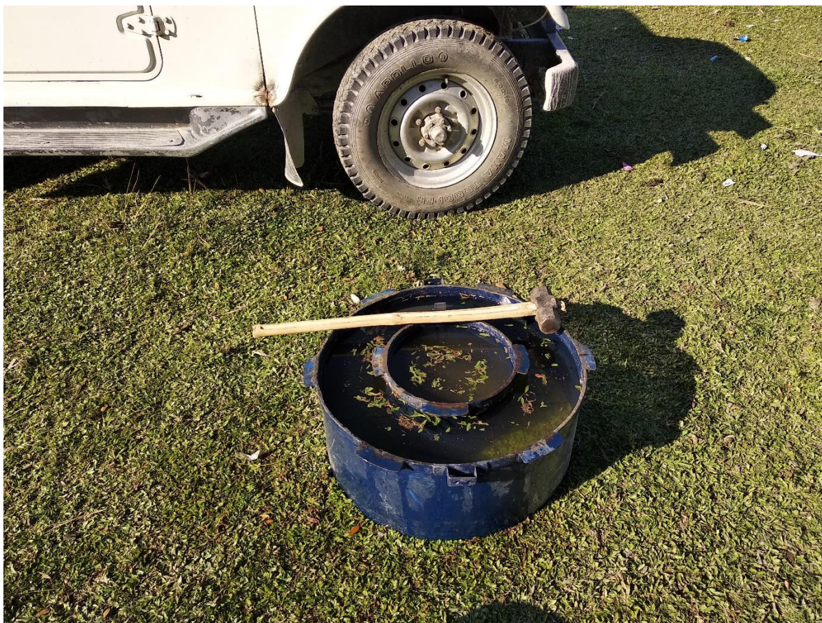
Field Photo 2.1 Soil Infiltration Test in progress
