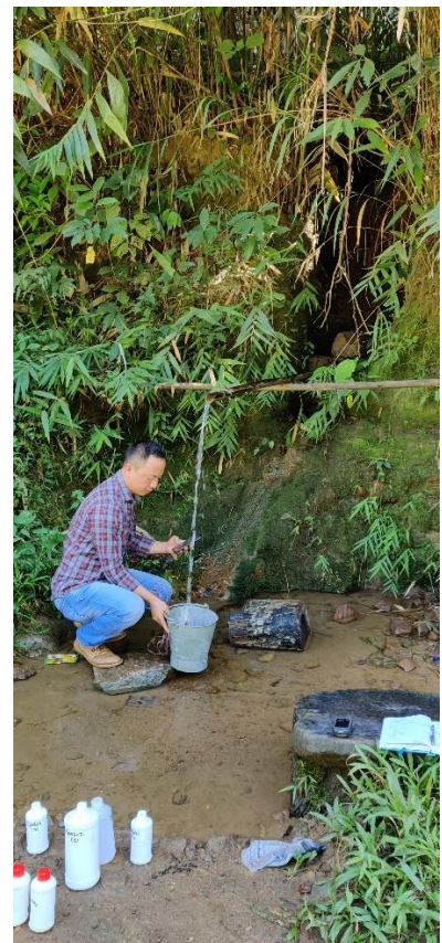
Spring discharge measurement and water sample collection in South Garo Hills district
