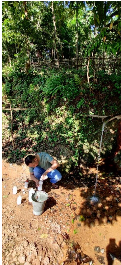
Spring discharge measurement and water sample collection in South Garo Hills district
