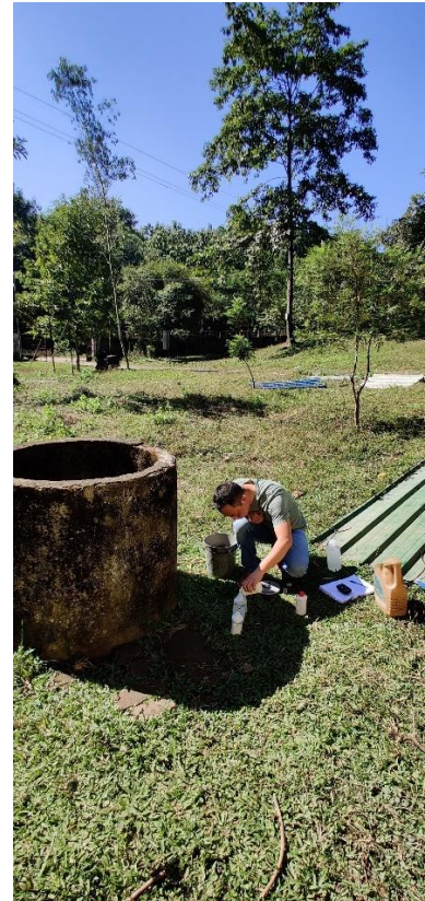
Water level measurement from dug well and water sample collection in South Garo Hills district
