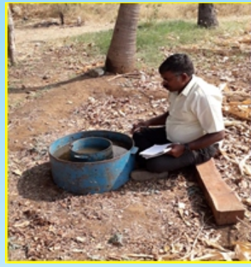
Infiltration Test conducted at Nachiyapuram, Andipatti block, Theni district, Tamil Nadu under Aquifer Mapping, Vaigai Basin, TN.
