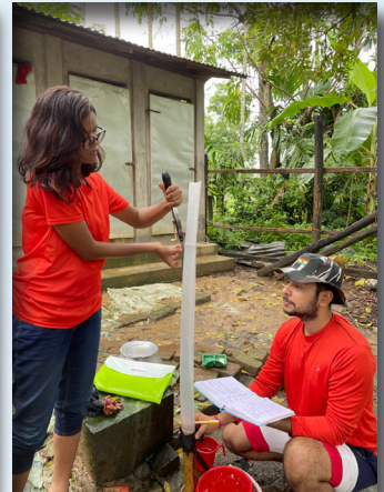
Monitoring of Piezometric Head at Khowai district, Tripura
