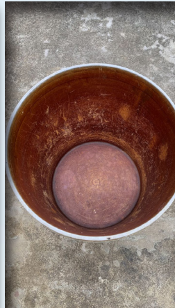
Iron encrustation at Char Ganki, Khowai block
