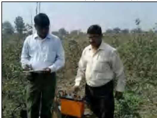
Geophysical Survey (in-House) VES by ABEM Terameter
