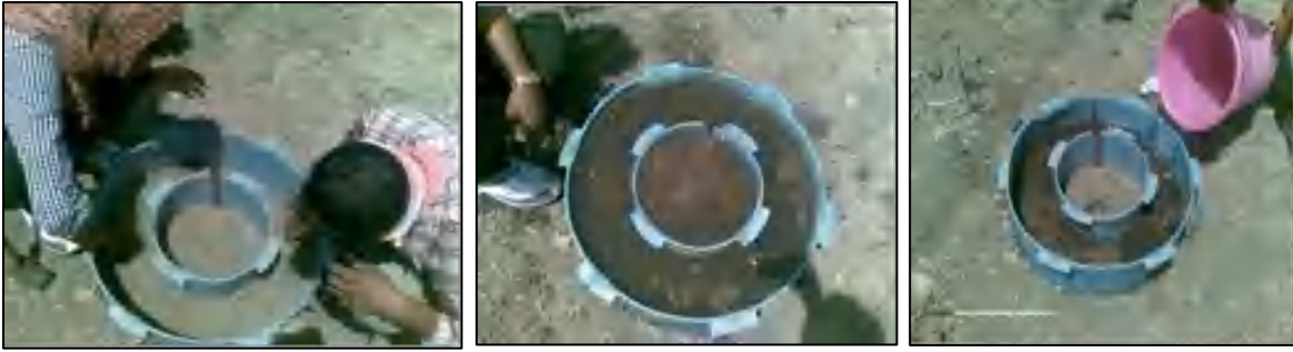
Double ring infiltrometer set up and collection of infiltration rate data.
