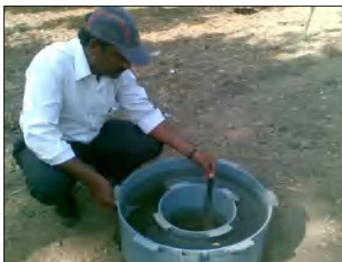
Fig.3.52: Field infiltration test, Chandrabhaga Watershed (WGKKC-2)
