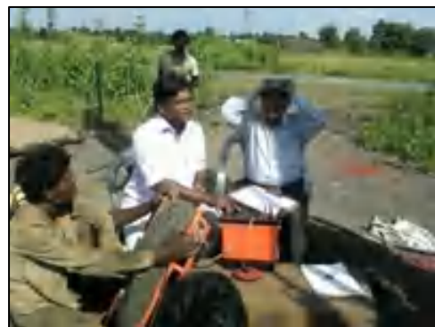
Geophysical Survey (in-House) VES by ABEM Terameter
