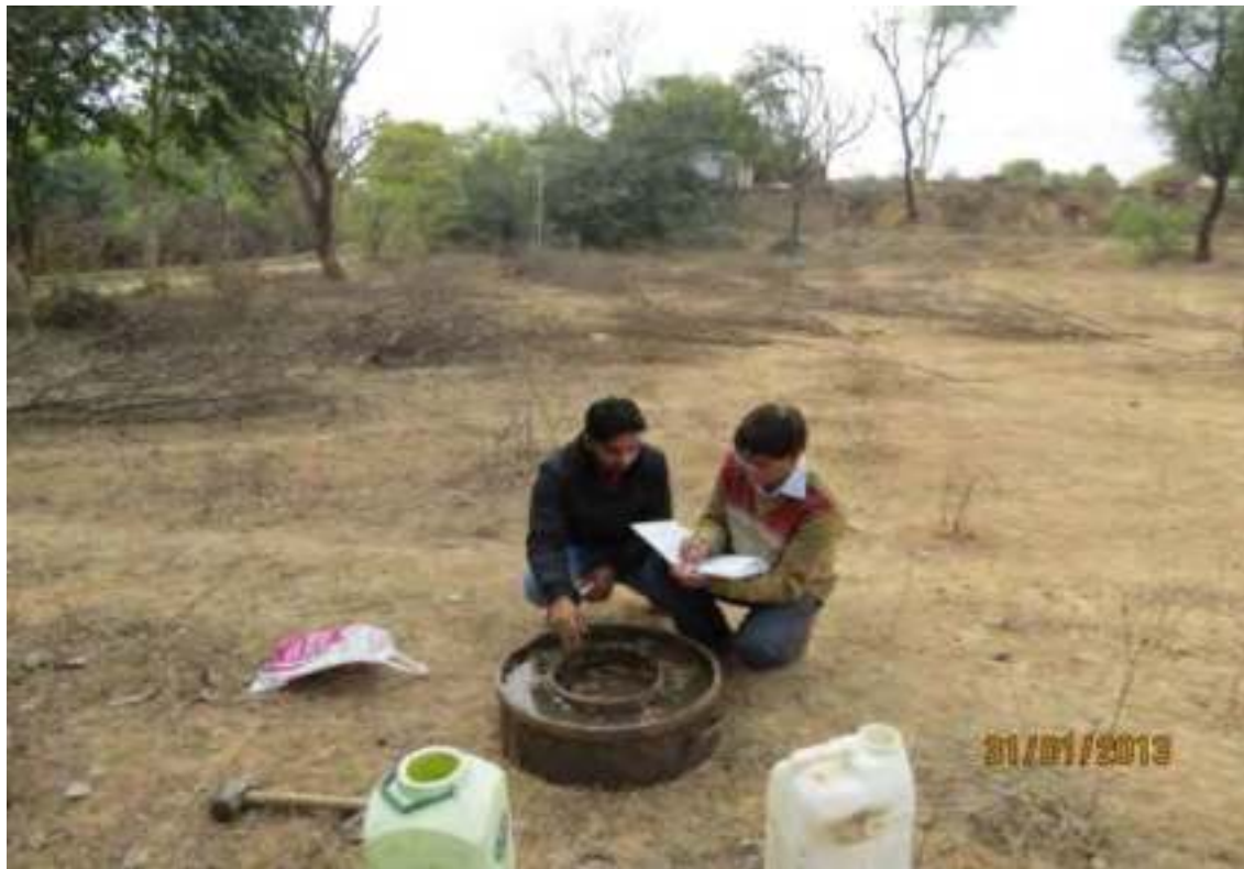
Plate 2. Soil Infiltration Test conducted in Baswa-Bandikui watershed
