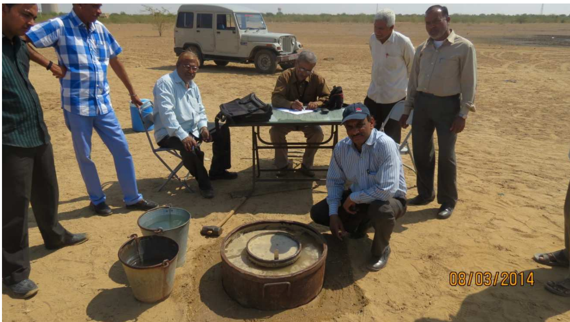
Plate 1. Soil Infiltration Test conducted in Ramgarh area, Jaisalmer district, Rajasthan
