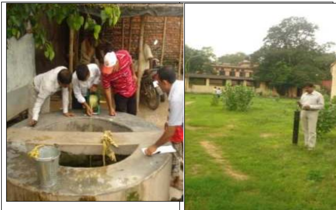
Fig 3.8 d: Field photograph showing (i) Groundwater level measurement in Dug well and (ii) Groundwater level measurement in piezometer.
