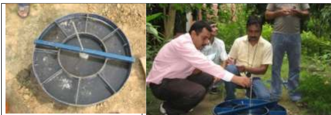
Fig 3.2 b : Infiltration rate test conducted in the field
