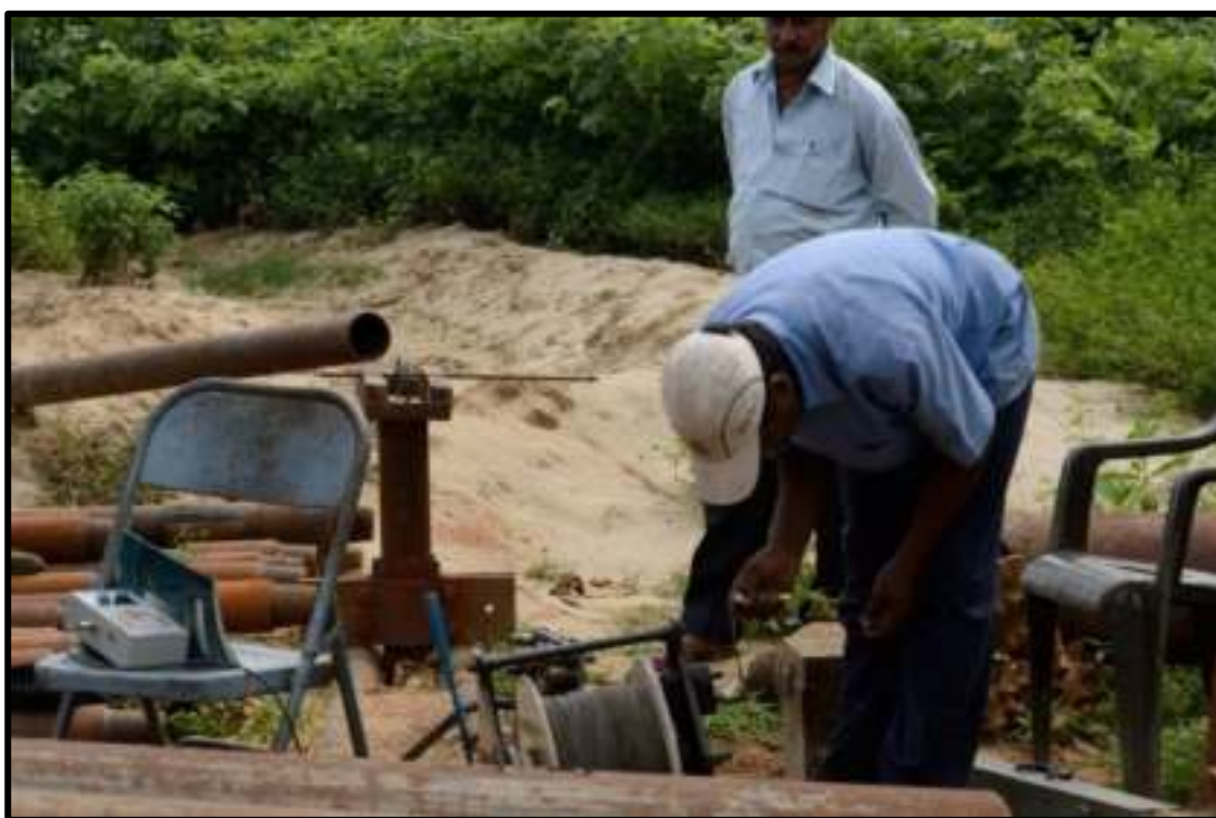
Fig: 3.13 b Field photograph showing gamma borehole logging carried out for radio-elemental concentration in the boreholes of the area
