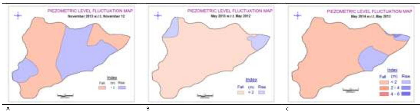
Fig 3.8 o: Annual Piezometric level fluctuation map (first aquifer) (i) Nov-12 to Nov.13 ( ii ) May-12 to May-13 ( iii ) May-13 to May-14
