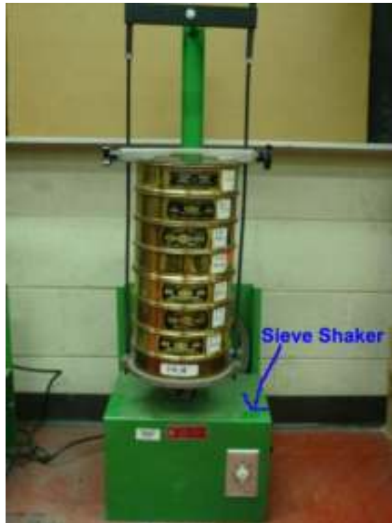
Fig 3.10 (c): Sieves shaker for grain size analysis
