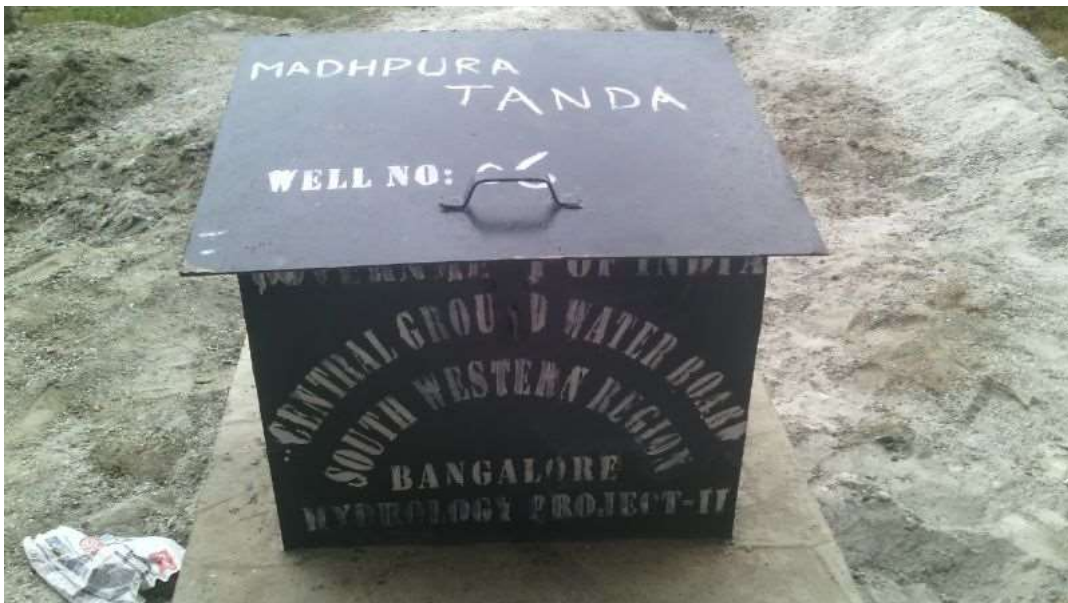
The exploratory well converted into piezometer for periodical monitoring
