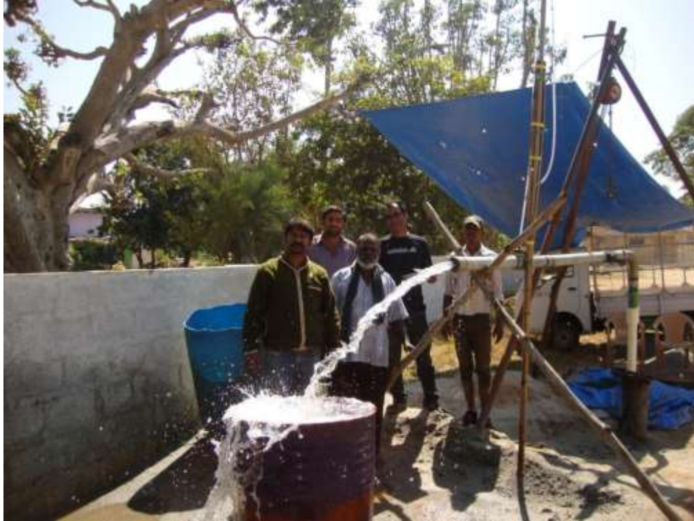
Long duration pumping test at Settikere EW site
