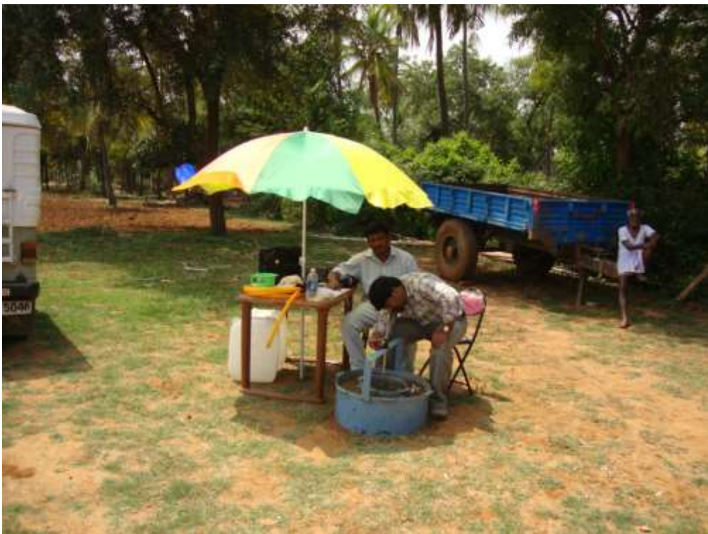
Double ring infiltration test at Rudrapura village
