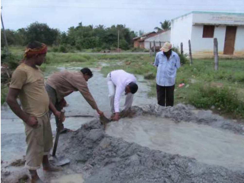
Measurement of drilling discharge through 90° V-Notch at Ankasandra EW site
