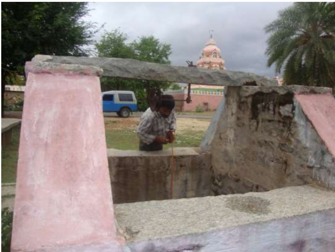
Measurement of ground water level in dug well at Halkurike village
