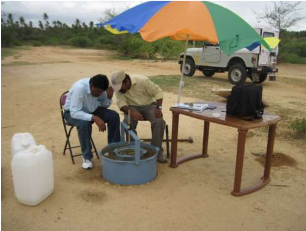
Double ring infiltration test at Bhairanayakanahalli village tank bed
