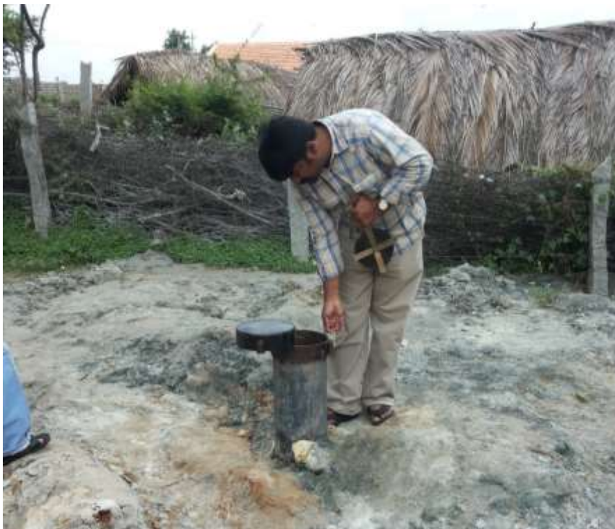
Measurement of ground water level in exploratory well at Huchanahatti EW site
