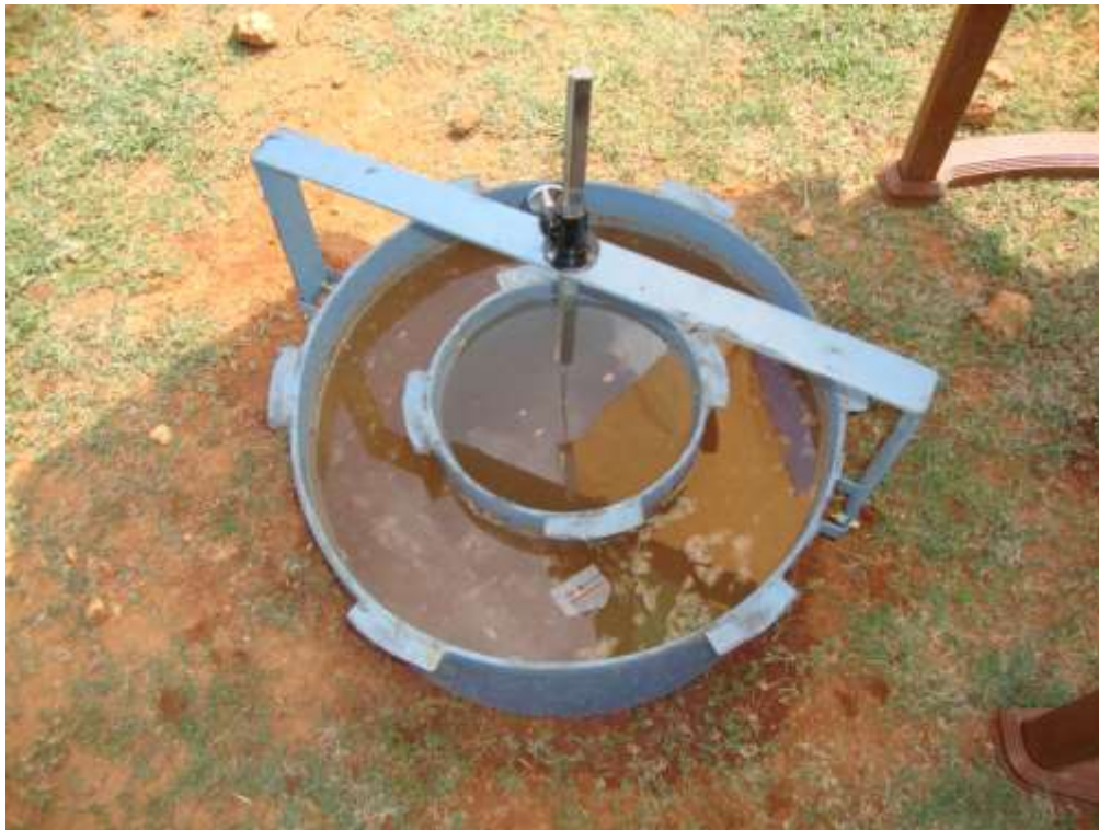
Double ring infiltration test at Misethimmanahalli village
