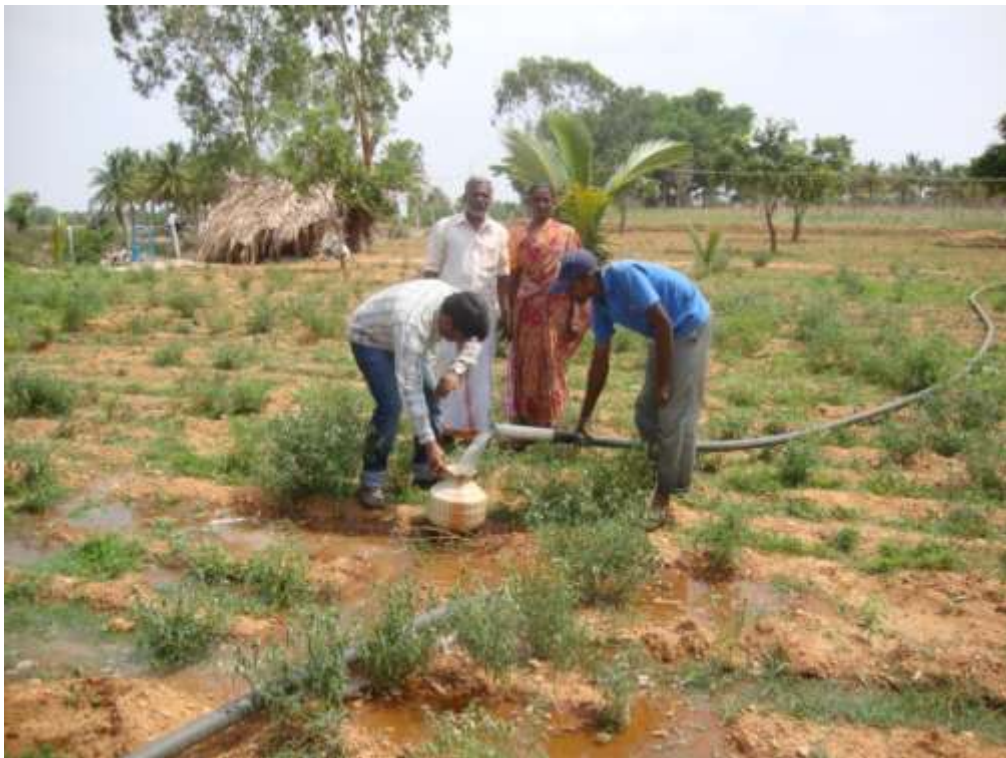
Measurement of discharge through volumetric method near Bommanahalli thanda village
