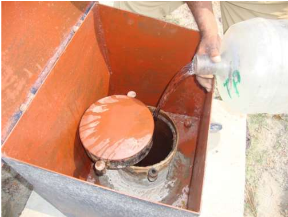
Slug test conducting at Bommanahalli thanda EW site
