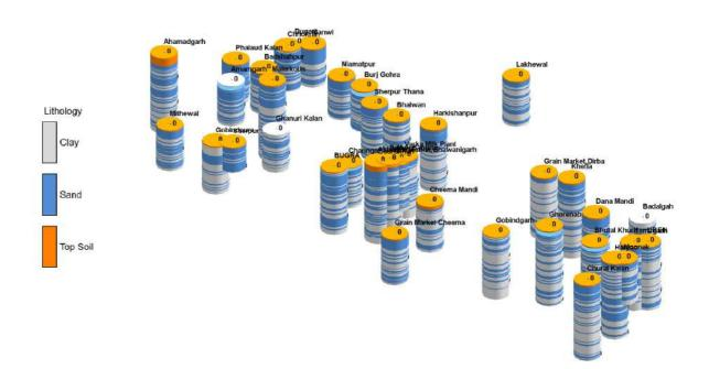
The data is validated by selecting the deepest well in each quadrant with those supported electrical logs for preparation of aquifer map and is shown below
