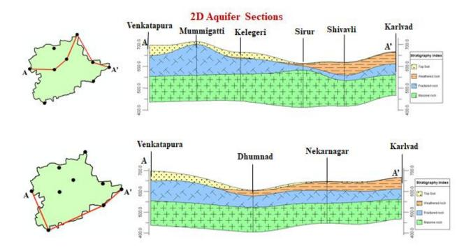
Fig.7: 2D Aquifer Cross Section, Dharwad taluk
