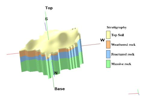
Fig.8: 3D Aquifer Disposition, Dharwad taluk
