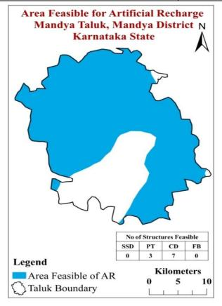
Fig.15: Area feasible for Artificial Recharge Structures
