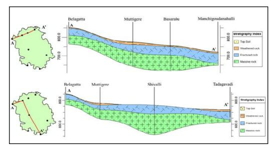
Fig. 13 (a) 2D Aquifer cross-section
