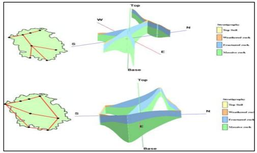
Fig.13(c): 3D Aquifer Fence Diagram
