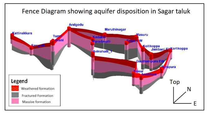
Fig. 3.3: Fence Diagramshowing aquifer disposition inSagarataluk
