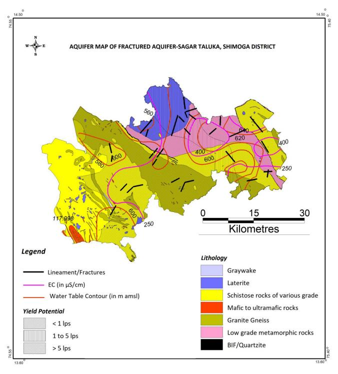
Fig. 3.7: Aquifer map of fractured aquifer system in Sagara taluk
