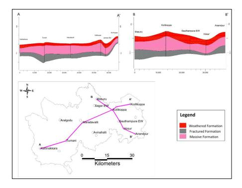
Fig. 3.2: Hydrogeological section taken along A-A' and B-B' of Sagara taluk
