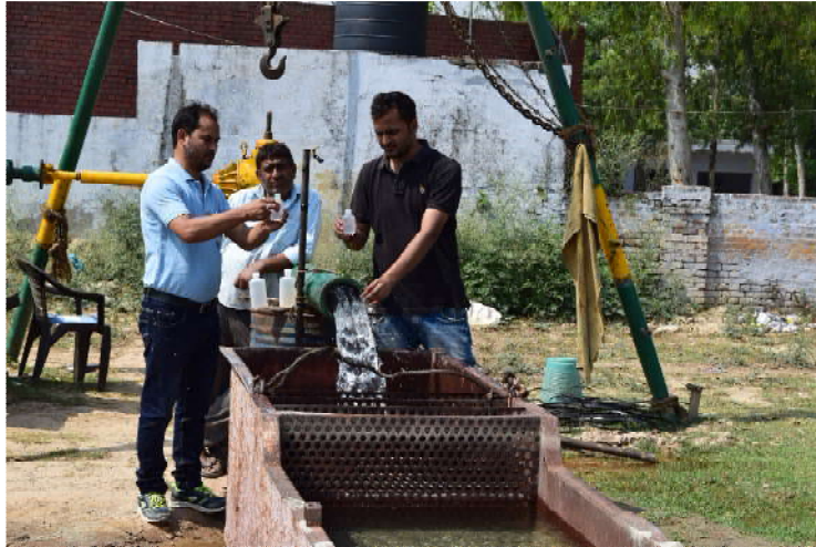
COLLECTION OF WATER SAMPLES DURING PUMPING TEST
