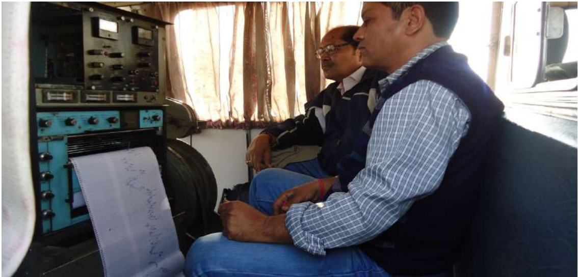
NATURAL GAMMA LOGGING, KURUKSHETRA (WELL FIELD)
