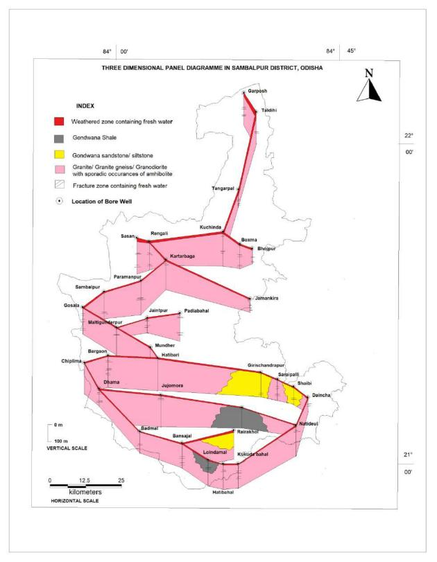
Fig.15a.Three-dimensional aquifer disposition model, Sambalpur District
