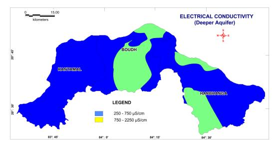
Fig. 3.5: Iso-conductivity Map of Fractured (Deeper) Aquifer.
