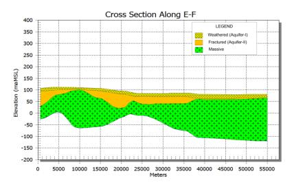
Fig. 3.14: Schematic Aquifer Cross-Section Along E-F in Boudh District.
