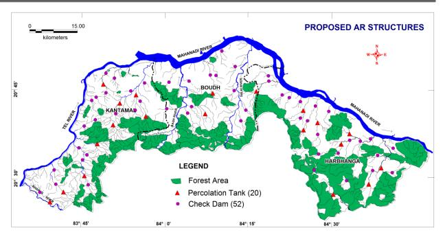
Fig. 5.2: Proposed sites for Artificial Recharge Structures.
