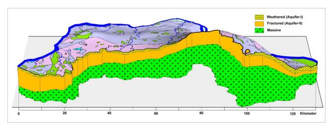
Fig. 3.10: Schematic 3D Aquifer Disposition in Boudh District.
