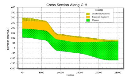
Fig. 3.15: Schematic Aquifer Cross-Section Along G-H in Boudh District.
