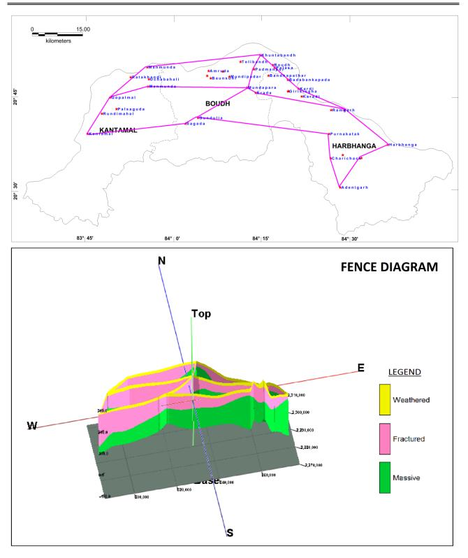
Fig. 3.17: Schematic 3D-Fence Diagram in Boudh District.
