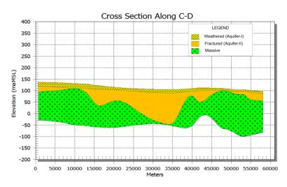
Fig. 3.13: Schematic Aquifer Cross-Section Along C-D in Boudh District.
