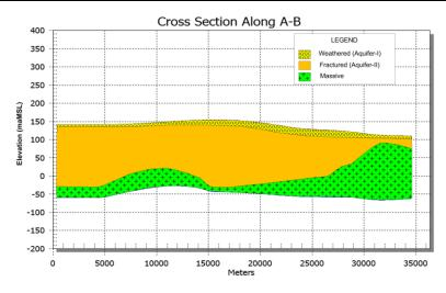
Fig. 3.12: Schematic Aquifer Cross-Section Along A-B in Boudh District.
