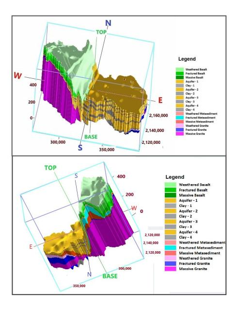
Fig.-3.17: 3-D Disposition of Aquifers
