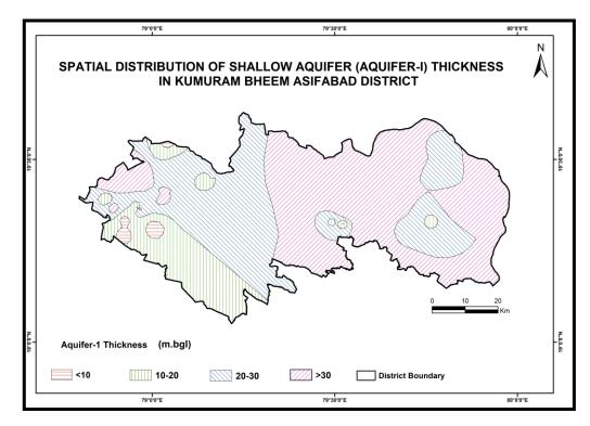
Fig. 3.15 : Spatial Distribution of Shallow Aquifer Thickness (Aquifer-1)
