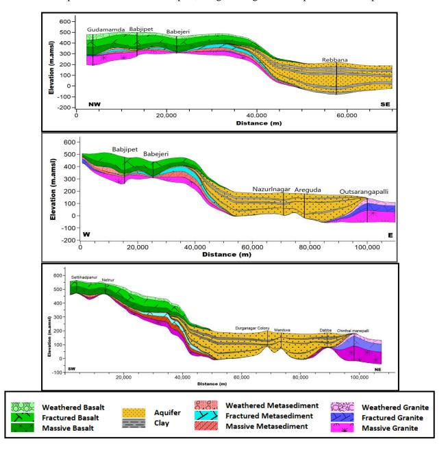
Fig.3.20 (a-c): Hydrogeological profile in different directions in Asifabad district.
