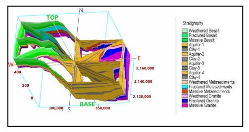
Fig.-3.18: Fence diagram
