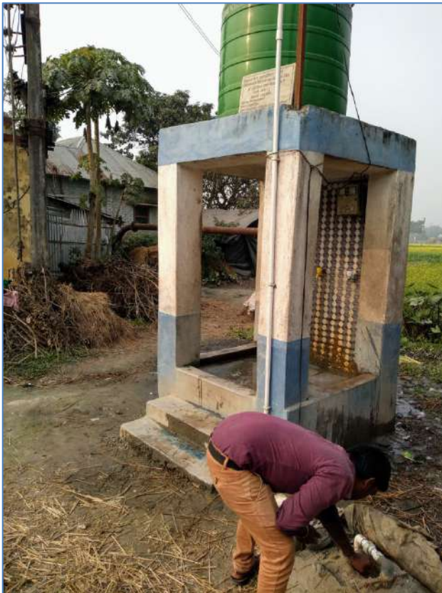
Measurement of water level in Key Observation Well established at Kanua, Chanchal-I block, Malda district during NAQUIM study (AAP: 2020-2021)
