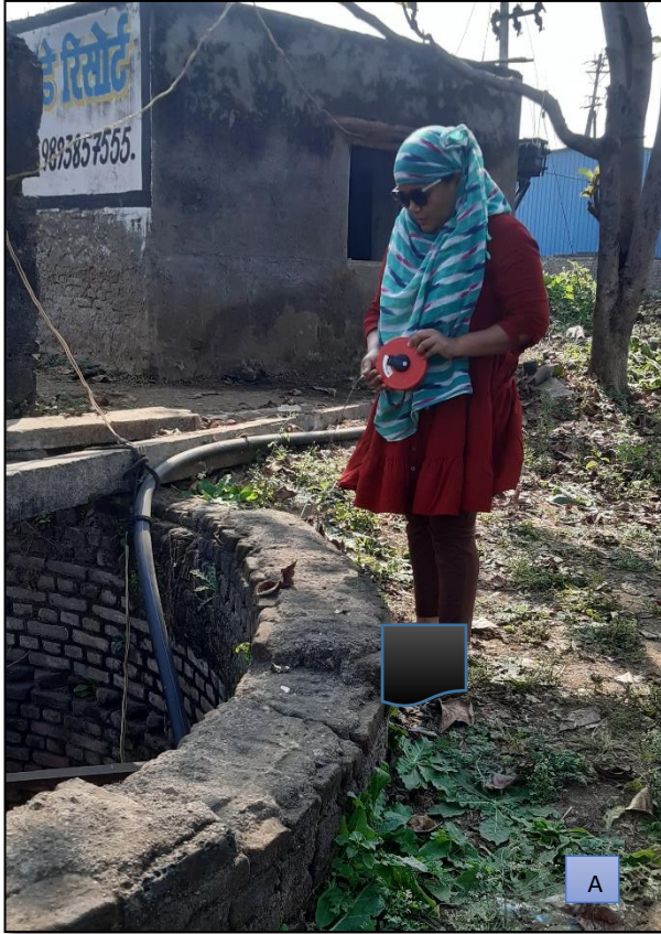
Figure 32 A & B Key Well Establishment and Water level monitoring
