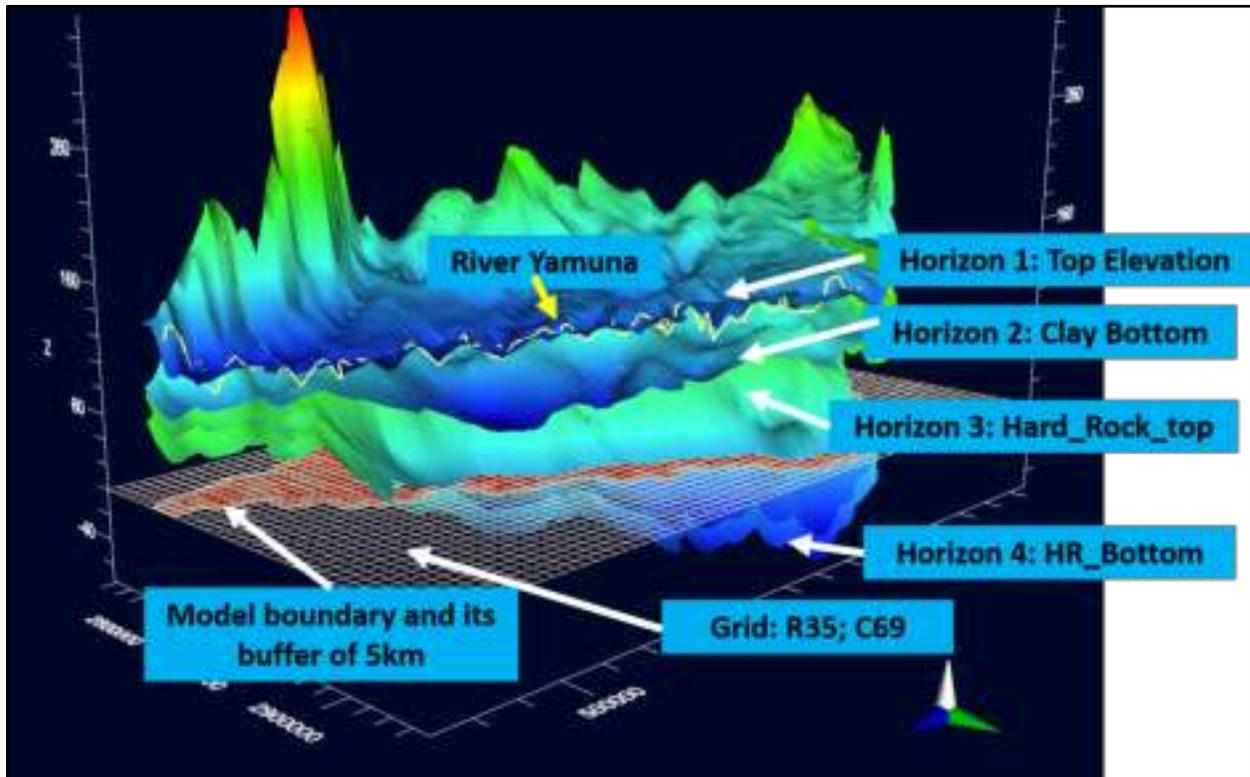
Figure 28: Horizontal extent of the model horizon with a 5km of boundary-buffer (Vertical exaggeration =500).
