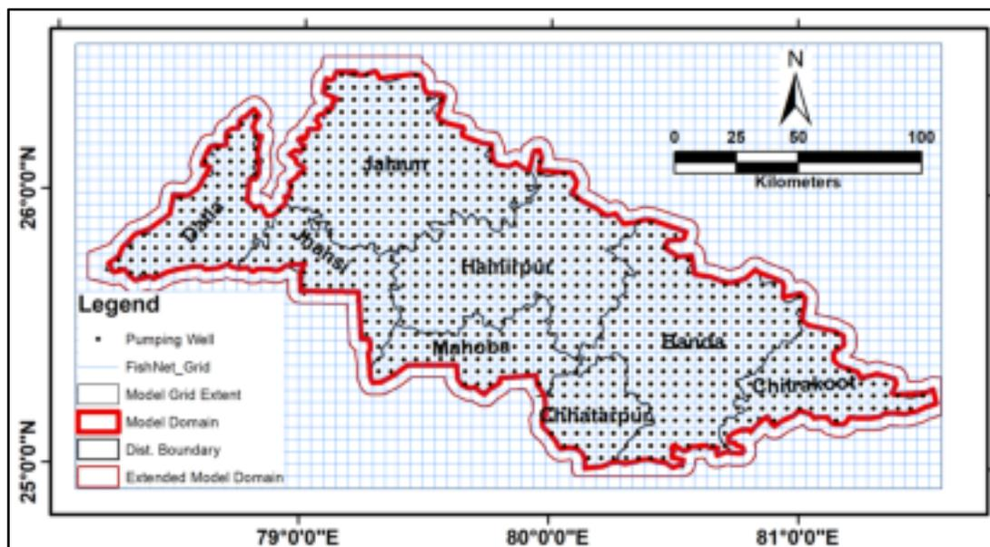
Figure 25: Generation of representative pumping well using Fish Net method in ArcGIS platform for the model input. A total of 857 representative pumping wells have been created in the model region.
