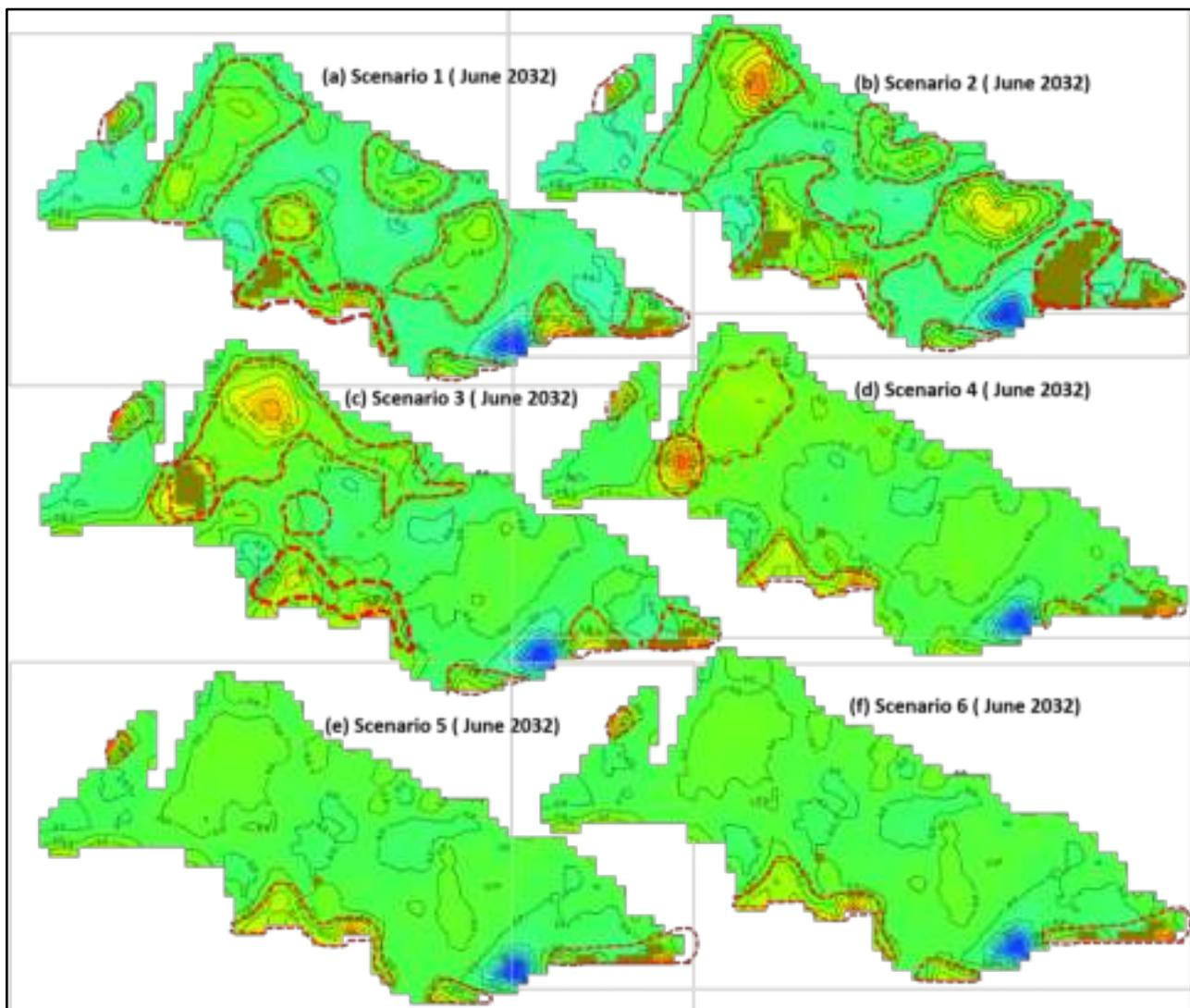
Figure 59: Summary of the probable hydrogeological condition after 15 years under different scenarios. The red broken line suggests the region to focus for implementing the AR and/or efficient irrigation under different scenarios.
