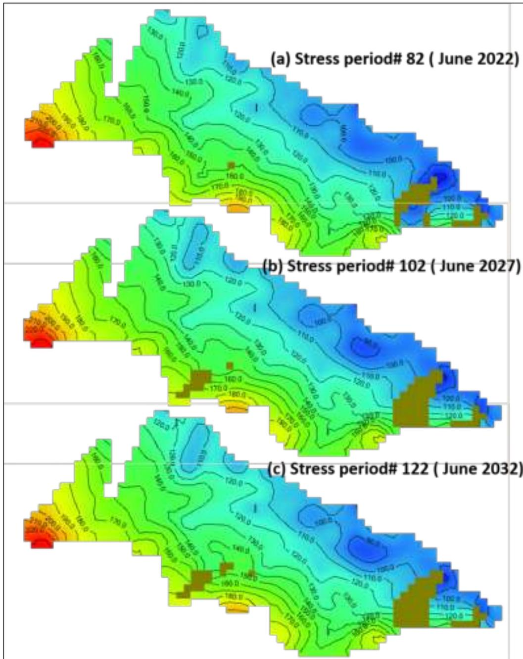
Figure 46: Water Level Map generated in Predictive Model Scenario – 2.
