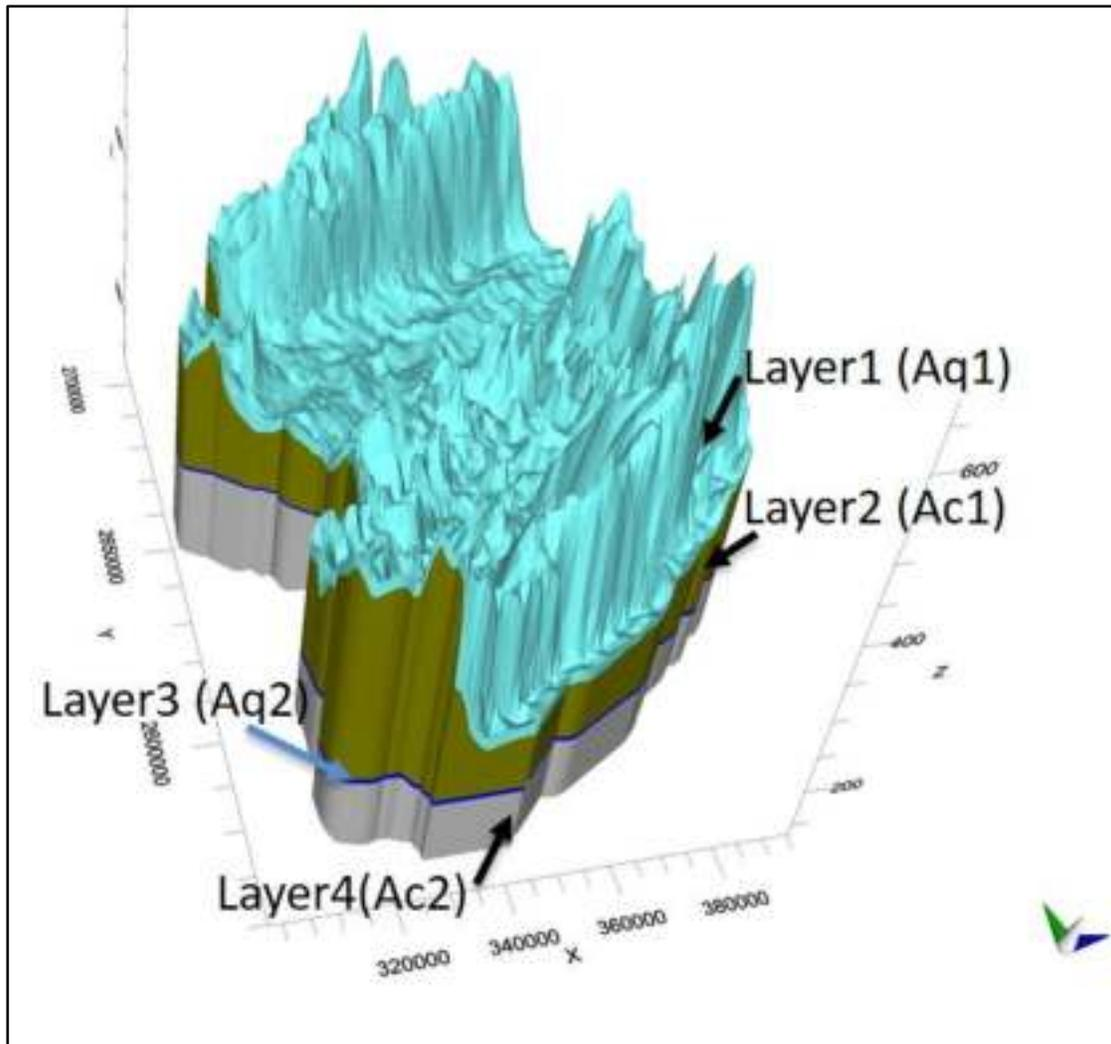
Figure 74: Conceptualization of different model layer using litholog data. (Vertical exaggeration =500).
