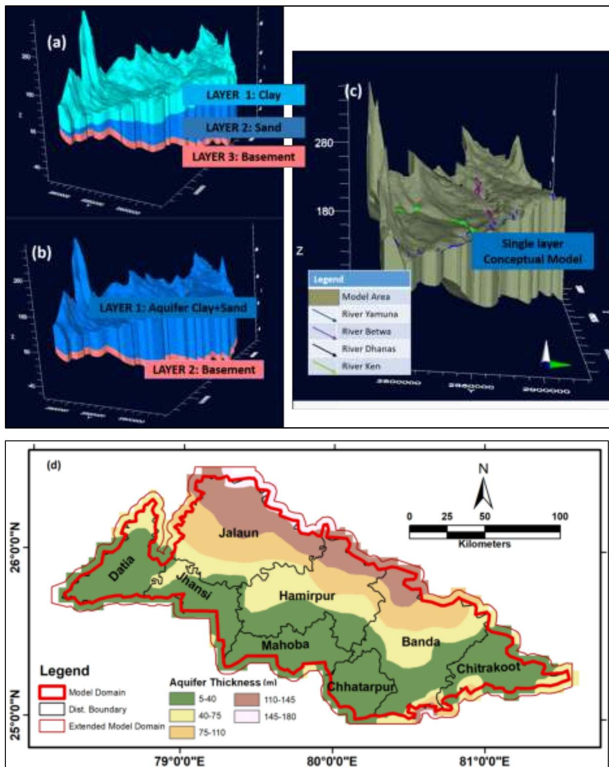
Figure 29: Development of a Conceptual model from three-layer to a single layer (a to c). A (Vertical exaggeration =500). Variation of the model thickness is plotted in figure 29 (d).
