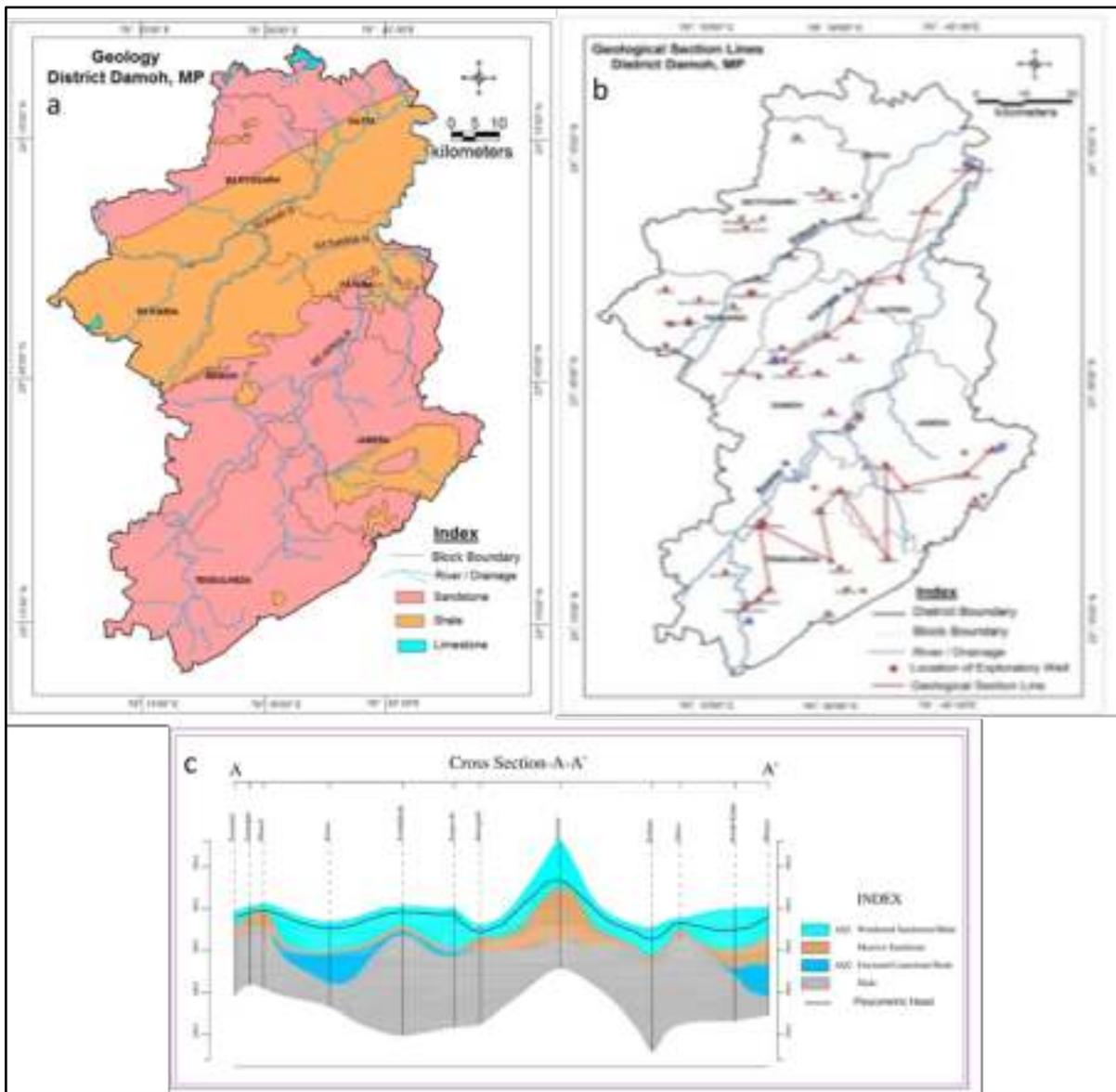
Figure 61: (a) Geological map, (b) location of lithological cross-section and (c) 2D cross-sectional profile along A-A' in the Damoh district. (Source: NAQUIM report, CGWB)
