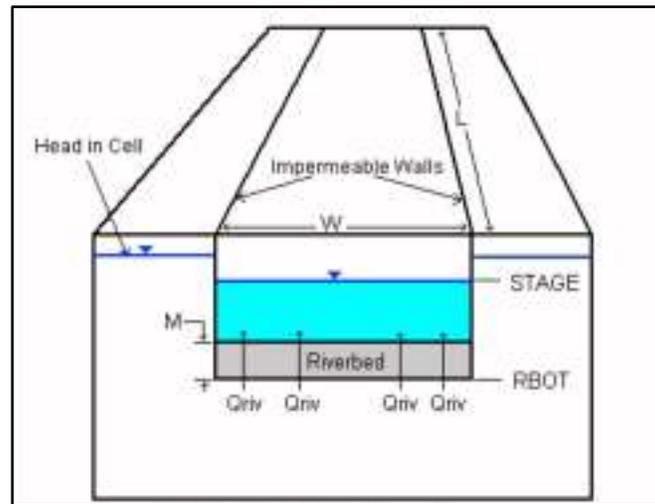
Figure 34: Schematic diagram of river boundary components (Source: [www.waterloohydrogeologic.com](http://www.waterloohydrogeologic.com))
