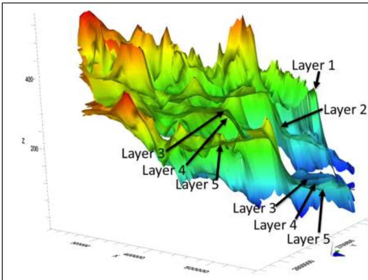
Figure 68: Different layers based on the CGWB lithologs. (Vertical exaggeration =500).
