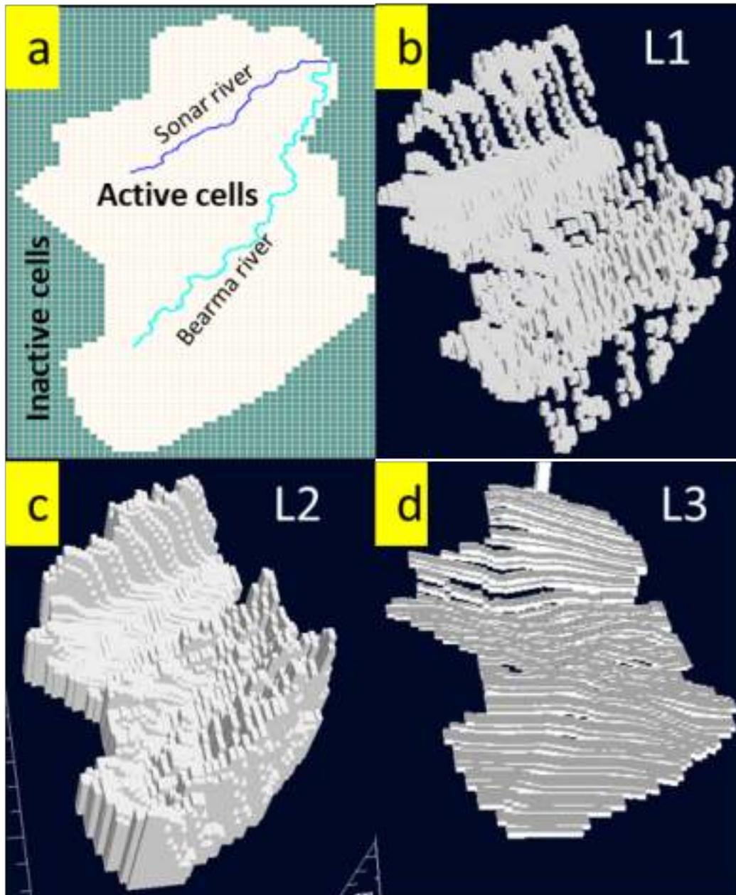
Figure 75: Defining the grids (a) layer view and (b, c, and d) 3D grid setting for layers 1, 2, and 3 after converting conceptual model (3-layer model) to a numerical model.
