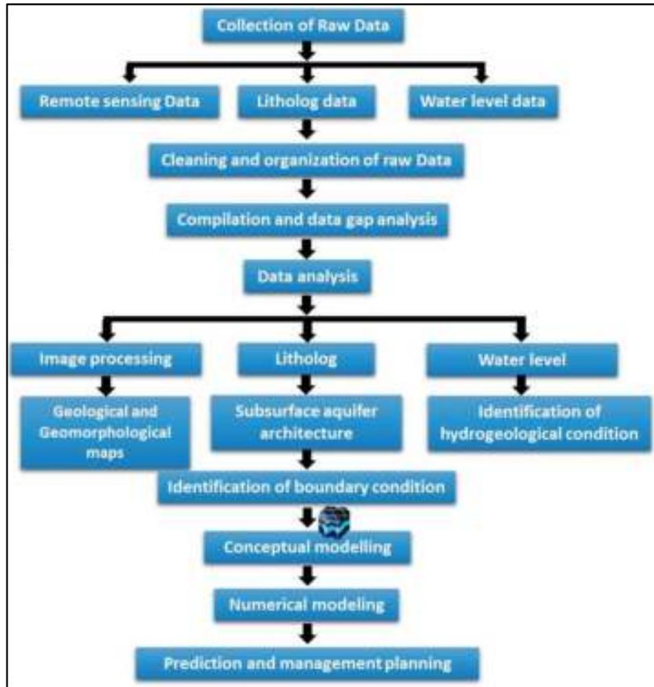
Figure 4: The major steps involved in data processing for flow modelling
