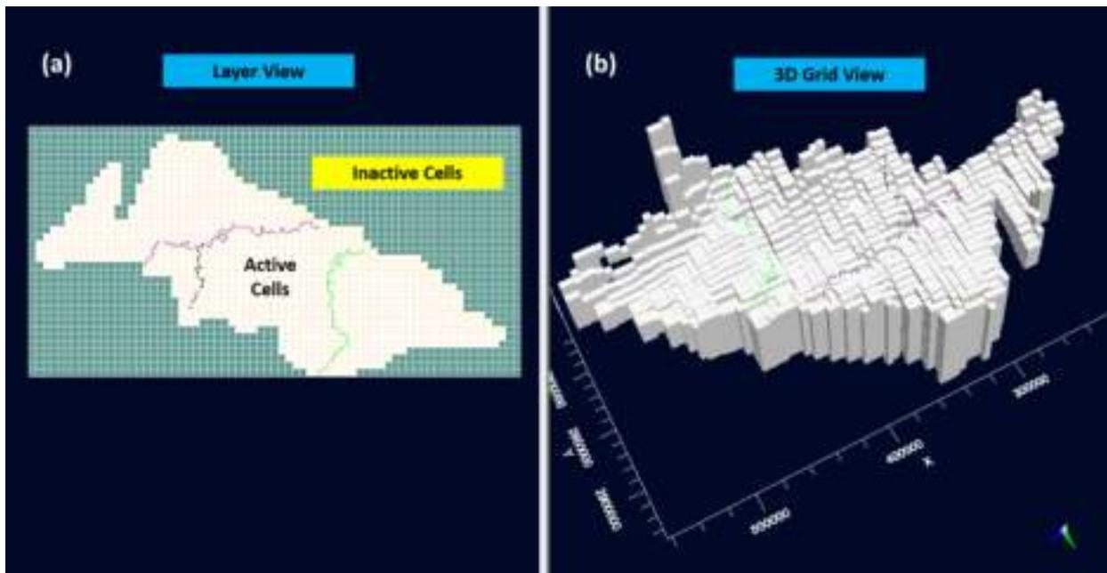
Figure 30: Defining the grids (a) layer view and (b) 3D grid for converting conceptual model to a numerical model.
