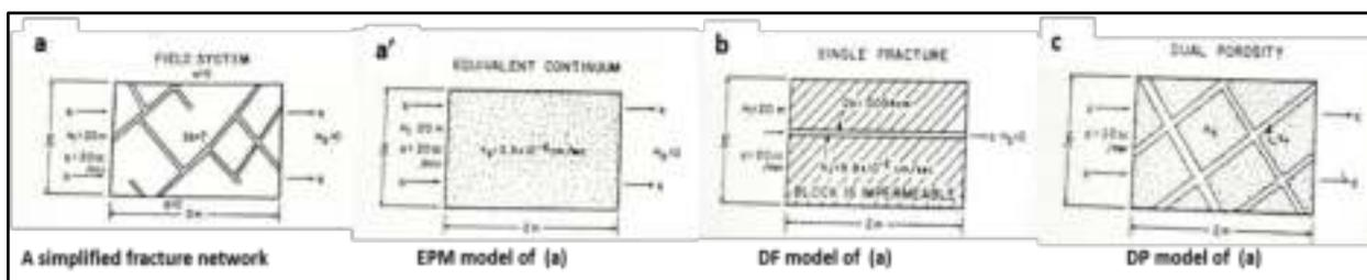
Figure 18: Representation of different conceptualisation methods of hard rock modelling.
