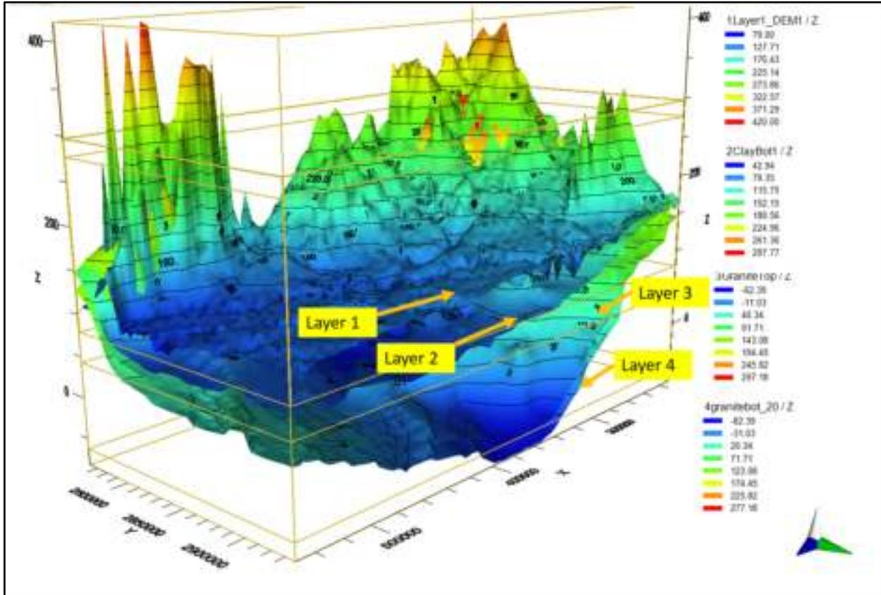
Figure 27: Different layers based on the CGWB lithologies. (Vertical exaggeration =500).
