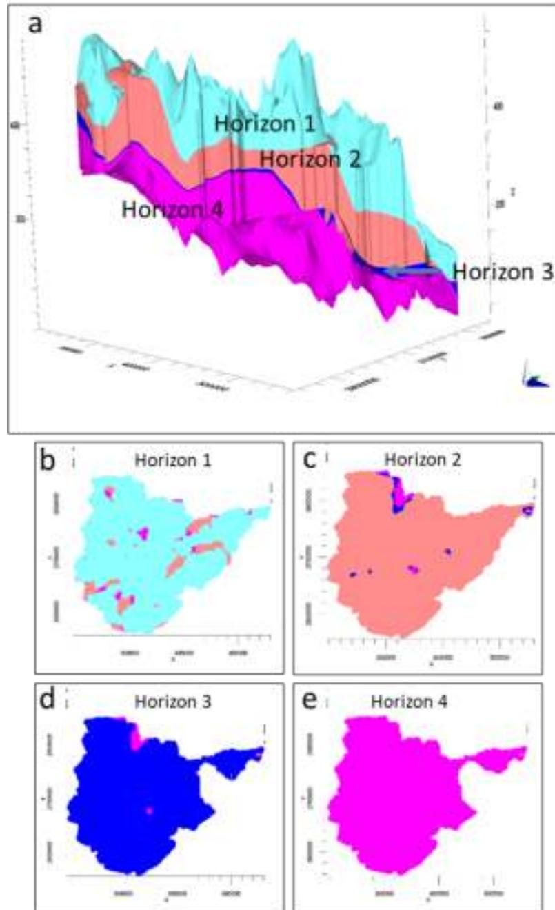
Figure 69: (a) Defining the horizons of the Bundelkhand Conceptual model for the hard rock terrain. (b) Horizon 1 intruded by horizon 2, (c) horizon 2 intruded by horizon 3 and 4, (d) horizon 3 intruded by horizon 4 (e) Horizon 4
