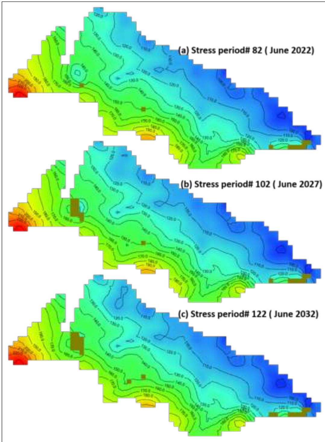
Figure 47: Water Level Map generated in Predictive Model Scenario – 3.
