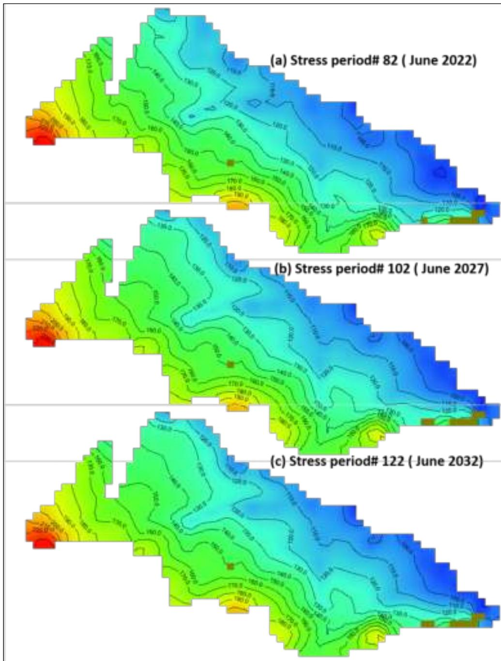
Figure 49: Water Level Map generated in Predictive Model Scenario – 5.
