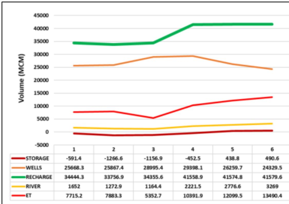
Figure 51: Different component of inflow and outflow for scenario 1 to 6.
