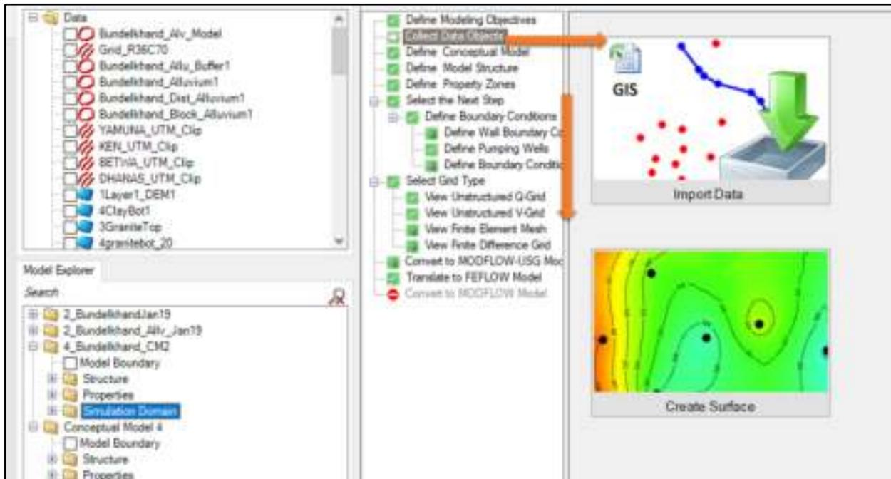
Figure 21: Workflow window for importing the various types of data in VMOD Flex.
