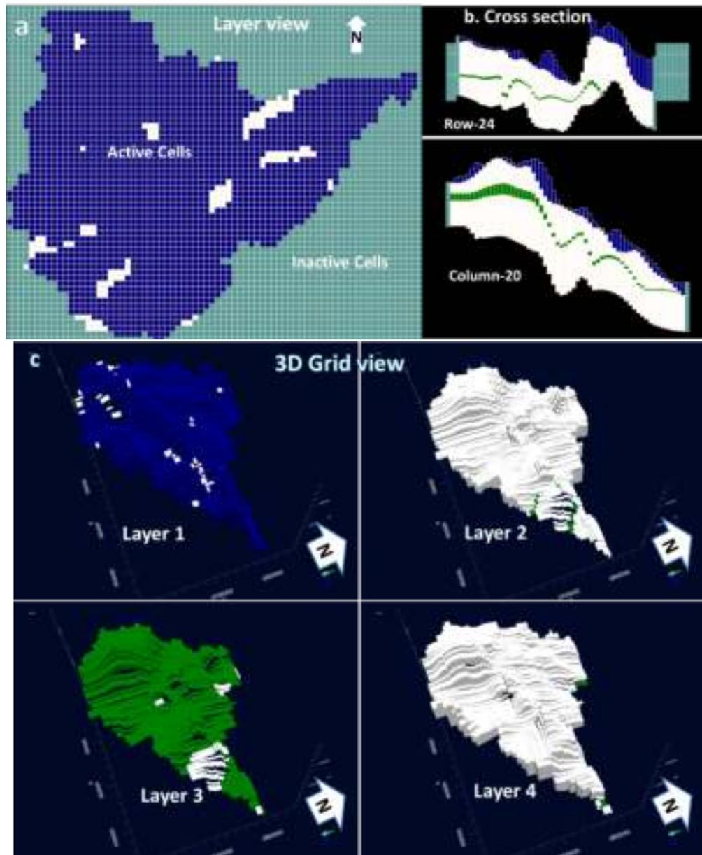
Figure 70: Showing the numerical grid in (a) Layer View, (b) cross-sectional view along row 24 and column 20, and (c) three-dimensional view of each layer.
