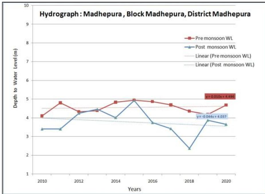
**Figure 13: Hydrograph Madhepura block**
