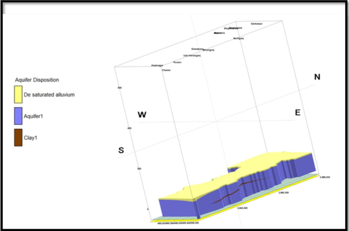
Figure 22: 3-D lithological and Aquifer Model
