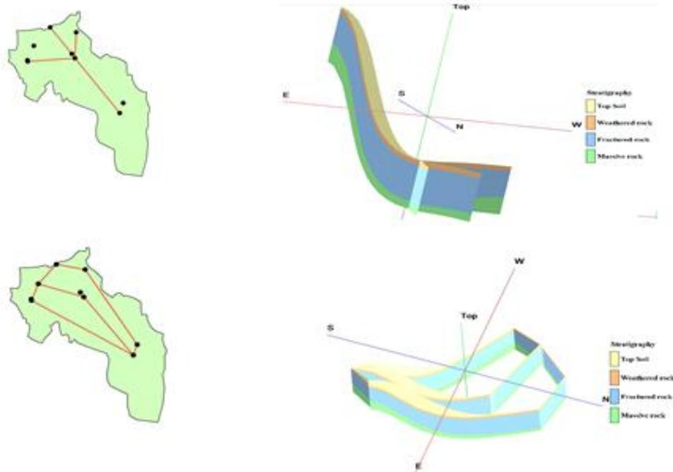
**Fig-10: 3D Aquifer Fence Diagram**
