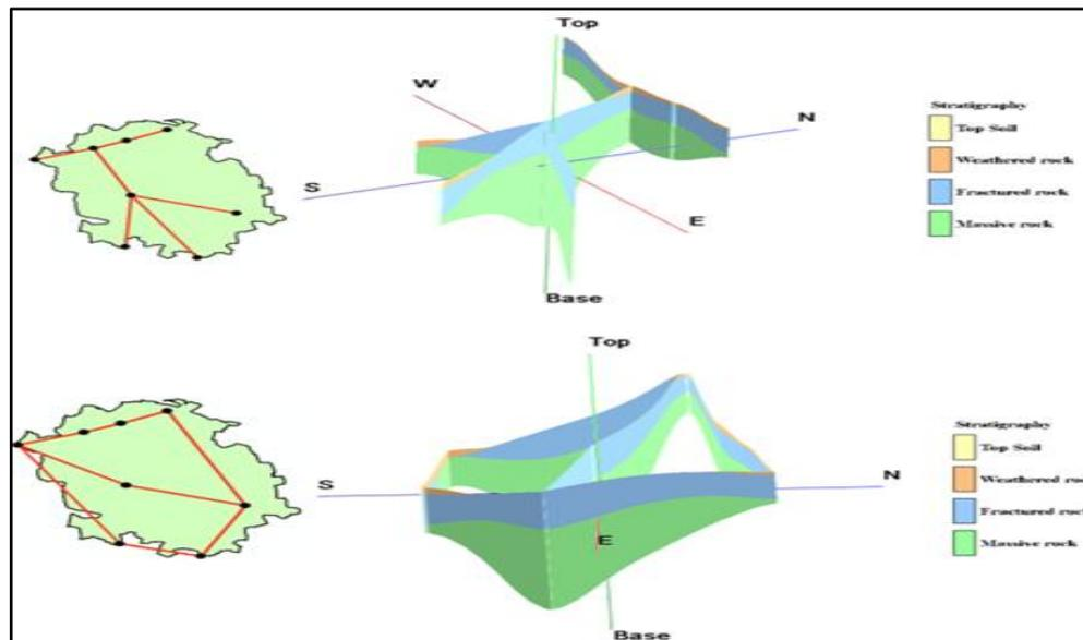
Fig.13(c): 3D Aquifer Fence Diagram
