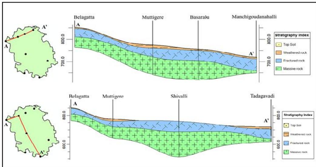
Fig. 13 (a) 2D Aquifer cross-section
