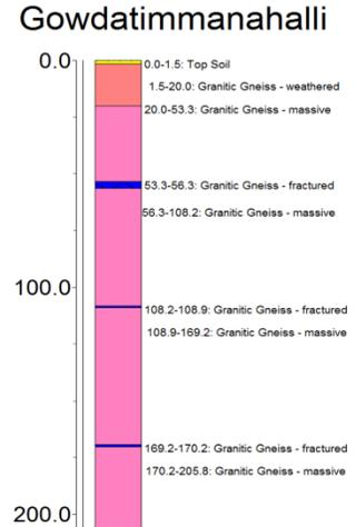
**Fig-12 Log diagram of Exploratory wells**
