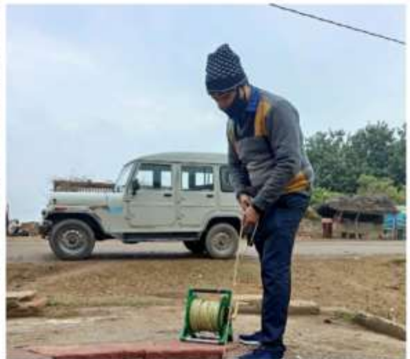
Figure 19: Field Photograph Showing Measuring Water level
