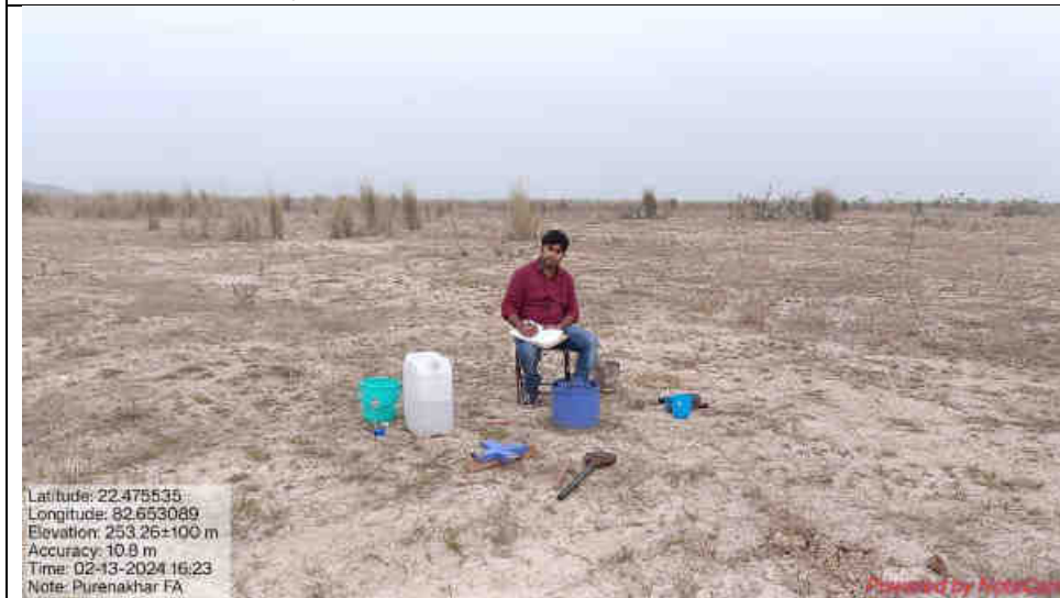
2. Soil Infiltration Test at Purenakhar Fly Ash Deposit Site
