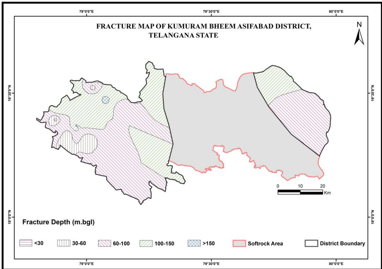
**Fig.3.16** : Spatial Distribution depth of fracture encountered in Hard Rock Area
