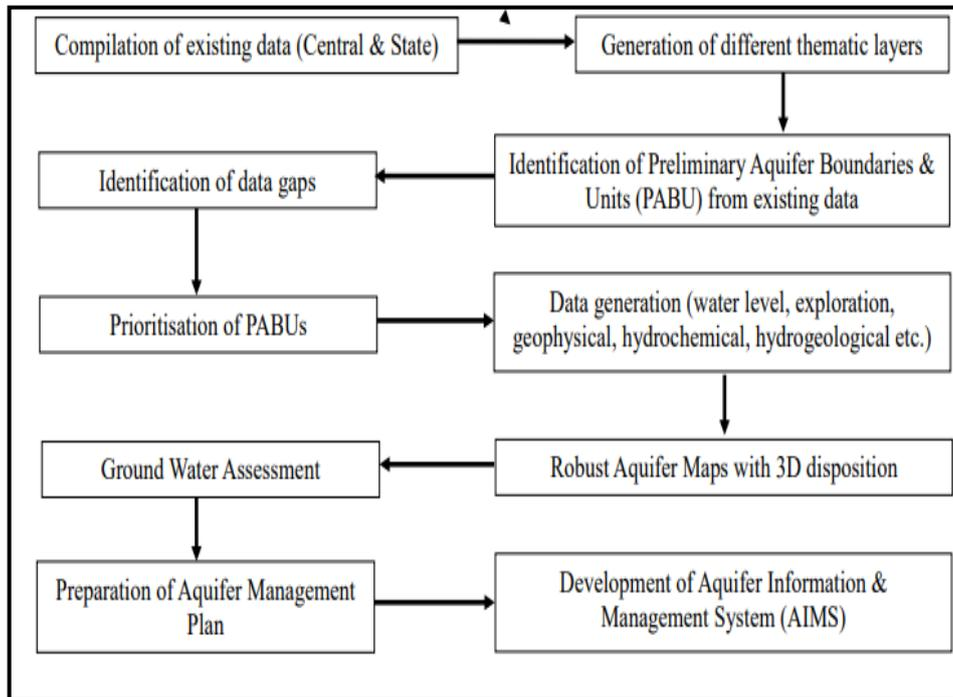
**Fig .1.1** : Action Plan of Aquifer Mapping
