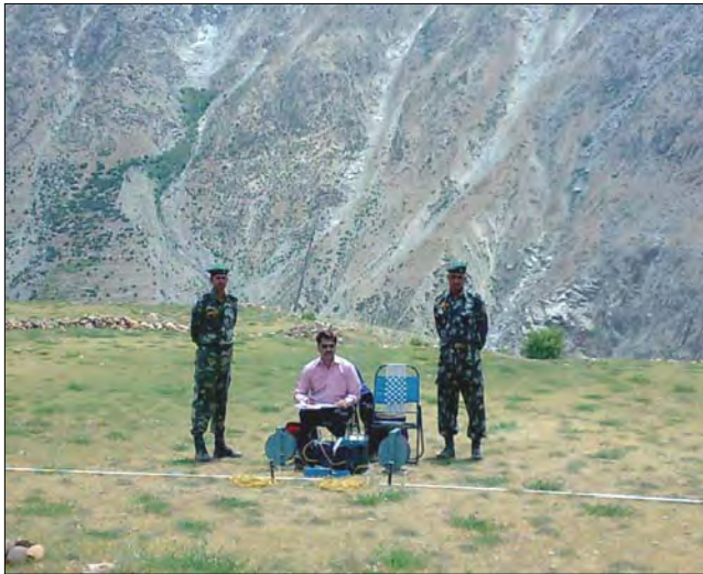
Fig. 9.1: Resistivity surveys in Kargil District were conducted at Kaksar Army Unit
