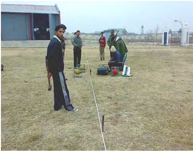
Fig. 9.2: Conducted VES at Snow & Avalanche Study Establishment (SASE) Rangreth (Srinagar) to pinpoint the site for construction of tubewell under short term water supply investigation
