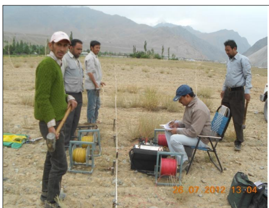
Fig 2.7 Resistivity Surveys at SKUAST, Kargil district (J&K)
