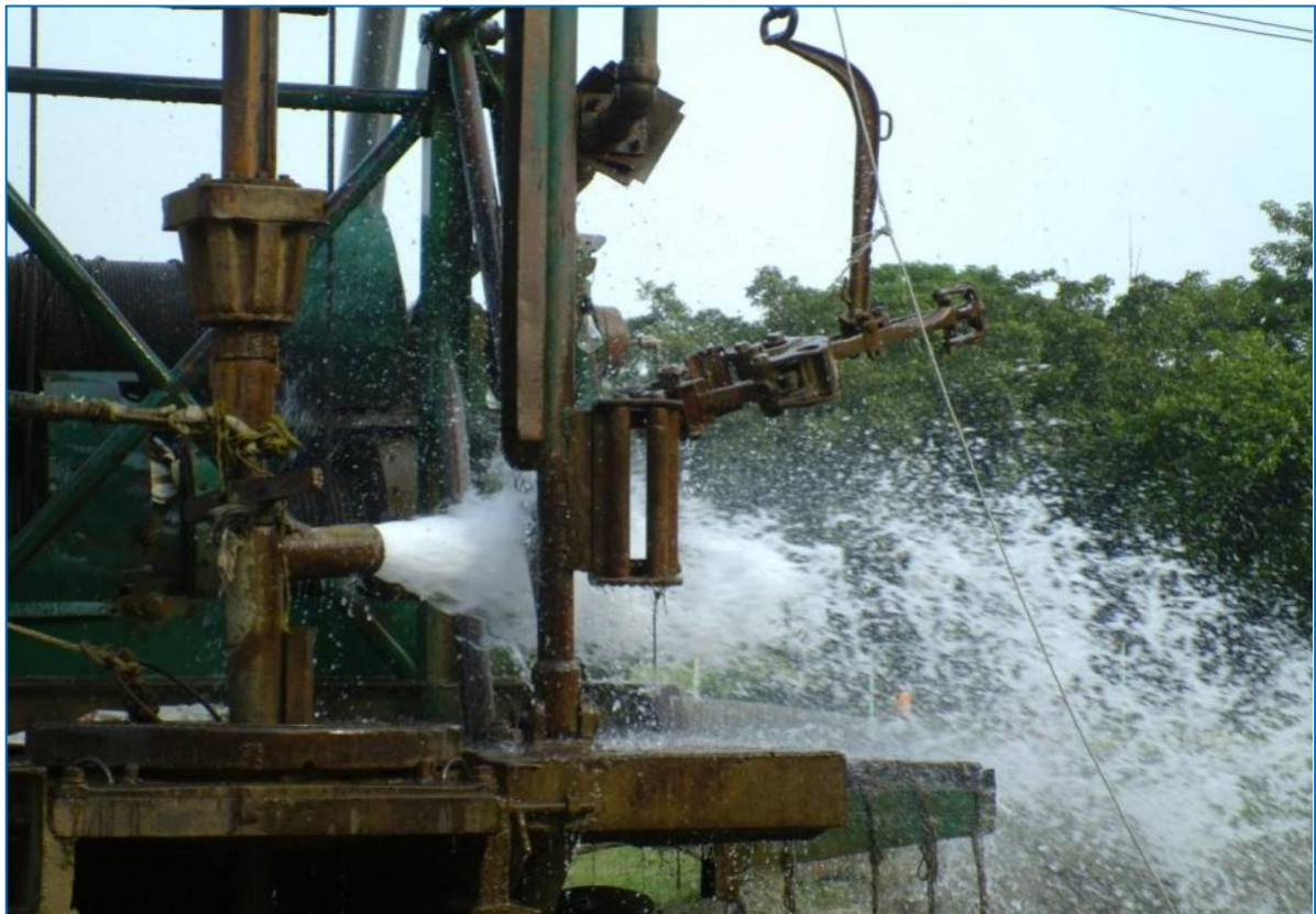
Fig 7.1: High yielding well at Chowgacha, Krishnanagar II block in Nadia district Discharge 1470 lpm
