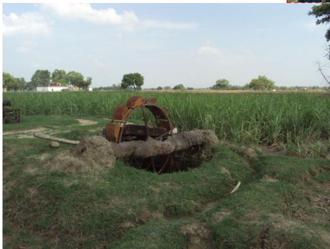
Plate 5: Rehat system for groundwater irrigation from dug well (at Amba) in Aurangabad district in the South Bihar Plain.
