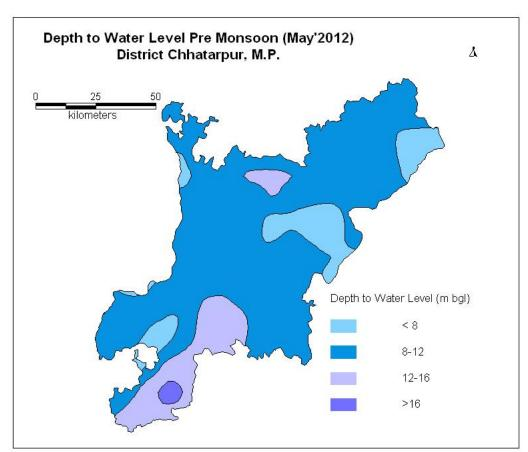
trend (2003-2012) shows declining trend ranges from 0.0015 to 0.64 m/year (Annual) water level fall is noticed in all block where a large scale withdrawal of ground water for irrigation purpose is observed (Fig-2).
