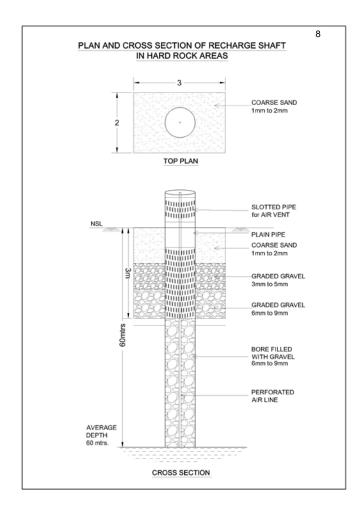
The opening for inflow to the well has been proposed at 1.5m above Bed level of pond. This is necessary to ensure that the pond retains sufficient water for use by local consumers. However, this may necessitate further deepening of pond itself so that the pond is 3-4 m deep. A Single well as discussed above would be suitable for a pond upto area of about 5ha. Therefore, more number of such Recharge wells is envisaged for larger ponds.
