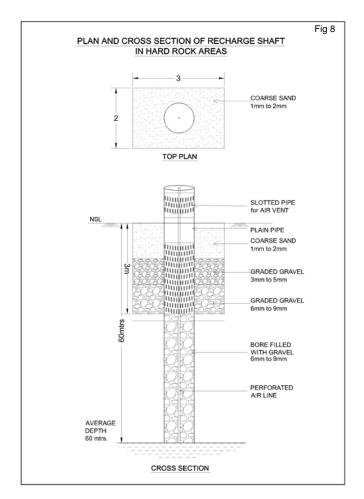
The model design of recharge well has been worked out in consultation with Ground Water Department, Government of Rajasthan and presented in Fig 8. The major features required are:
