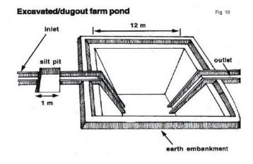
soil, the farmer's water requirements, the cost of excavation, and the possible uses of the excavated earth. Water from the farm pond is conveyed to the fields manually, by pumping, or by both methods. Pictorial diagram of farm pond is shown in fig 10.
