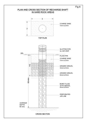
The model design of recharge well has been worked out in consultation with Ground Water Department, Government of Rajasthan and presented in Fig 8. The major features required are:
