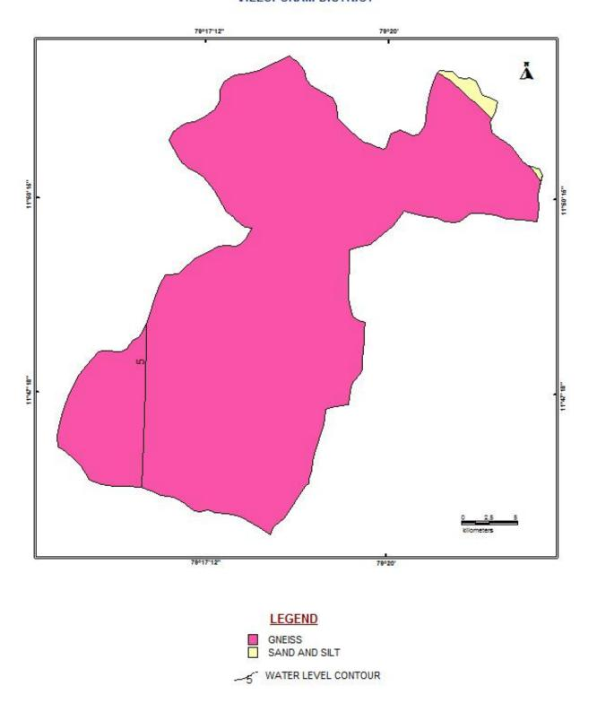
Figure 5. Hydrogeological Map of Kalamarudur Firka
