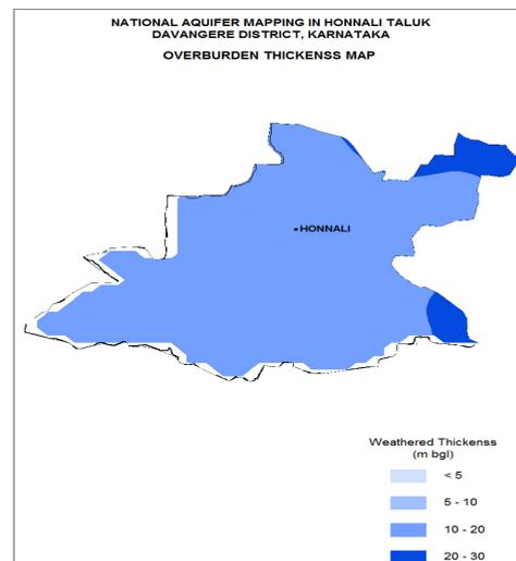
Figure-11: Weathered Thickness Map
