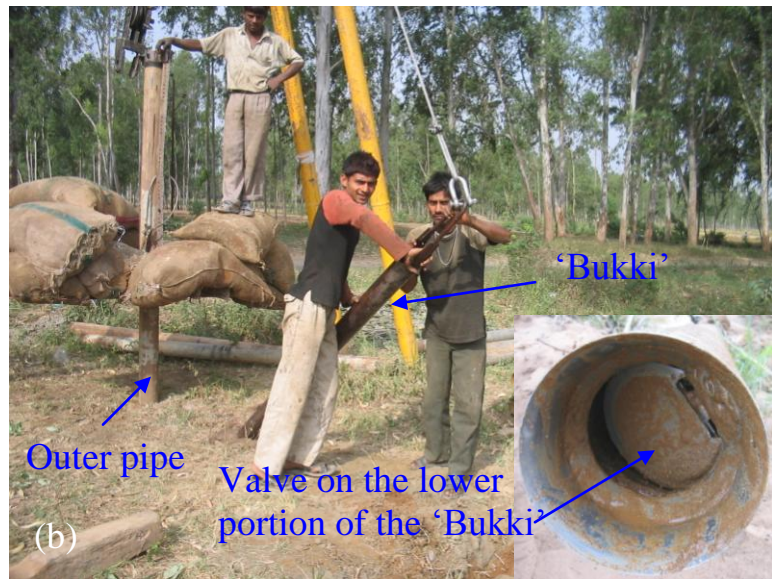
Figure 7.1: Drilling conducted on the paleochannel near Berla village. (a) Machine operated 'Bukki System' and (b) Different parts of 'Bukki System'.
